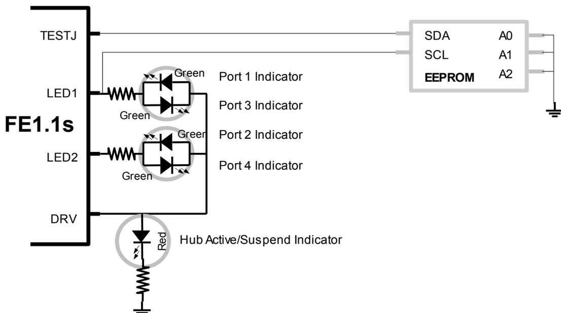
Fig. 3: LED and EEPROM Connections
