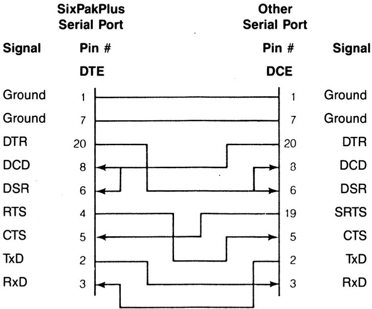
**Figure B-4. Example #3: Null Modem Interface.**
