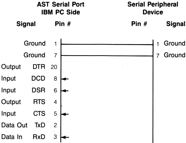
**Figure B-5. Serial Interface Form.**
