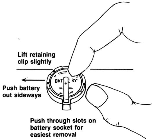
**Figure 3-2. Removing the SixPakPlus Clock/Calendar Battery.**
