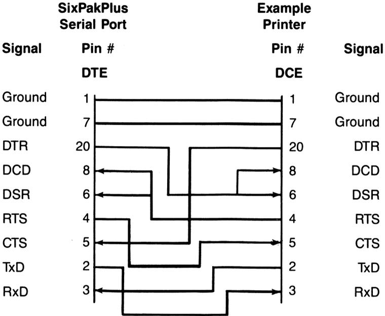
**Figure B-3. Example #2: Null Modem Interface.**
