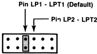
NOTE: When IBM or AST Monochrome Card is installed, SixPakPlus LPT1 automatically responds as LPT2, and SixPakPlus LPT2 automatically responds as LPT3.
