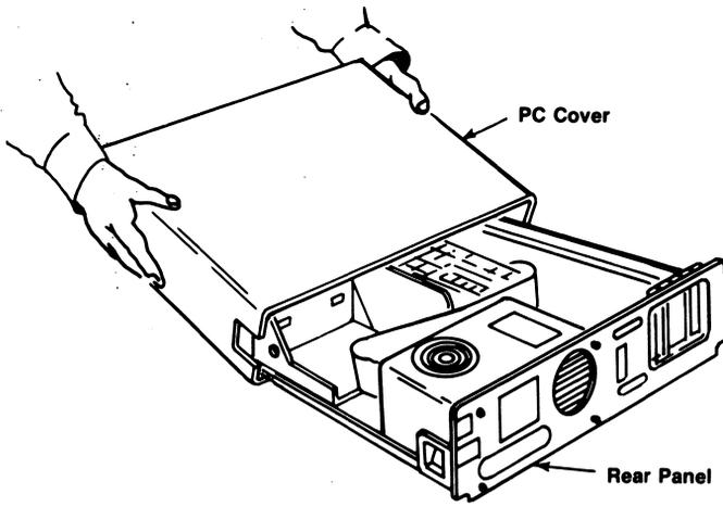
**Figure 2-7. Removing the PC Cover.**
