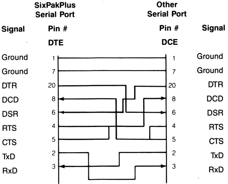
**Figure B-2. Example #1: Null Modem (DTE-to-DTE) Interface.**
