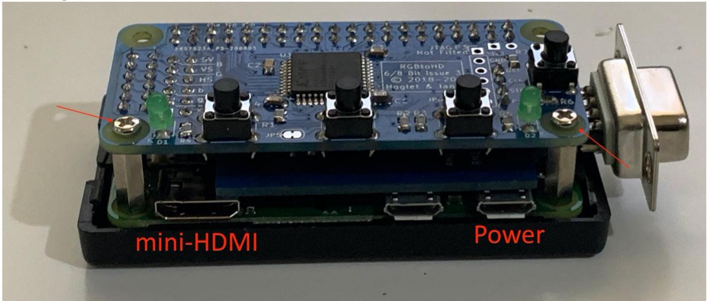
**Note:** Please make sure you only power your RGBi to HDMI Video Processor via the Micro-B connector closest to the Video Input connector. Using the other port has been known to kill SD cards.
