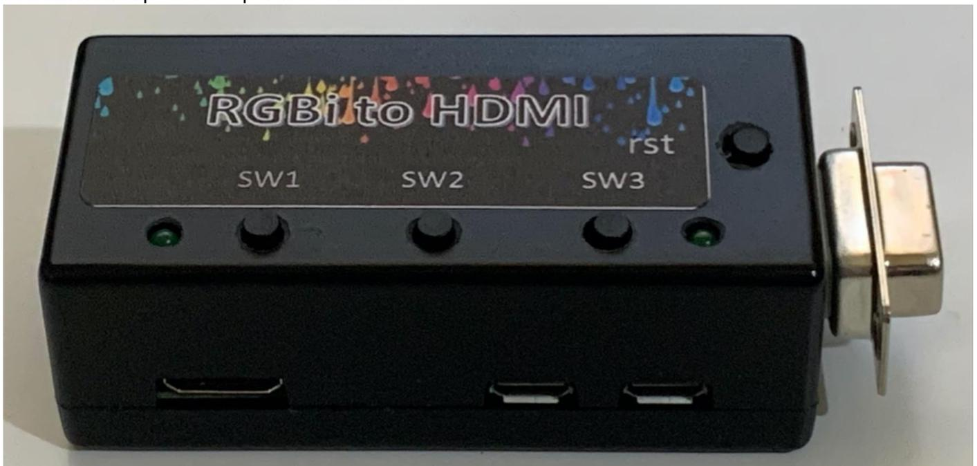
**Note:** The case clips can be fragile and break if taken apart multiple times.
