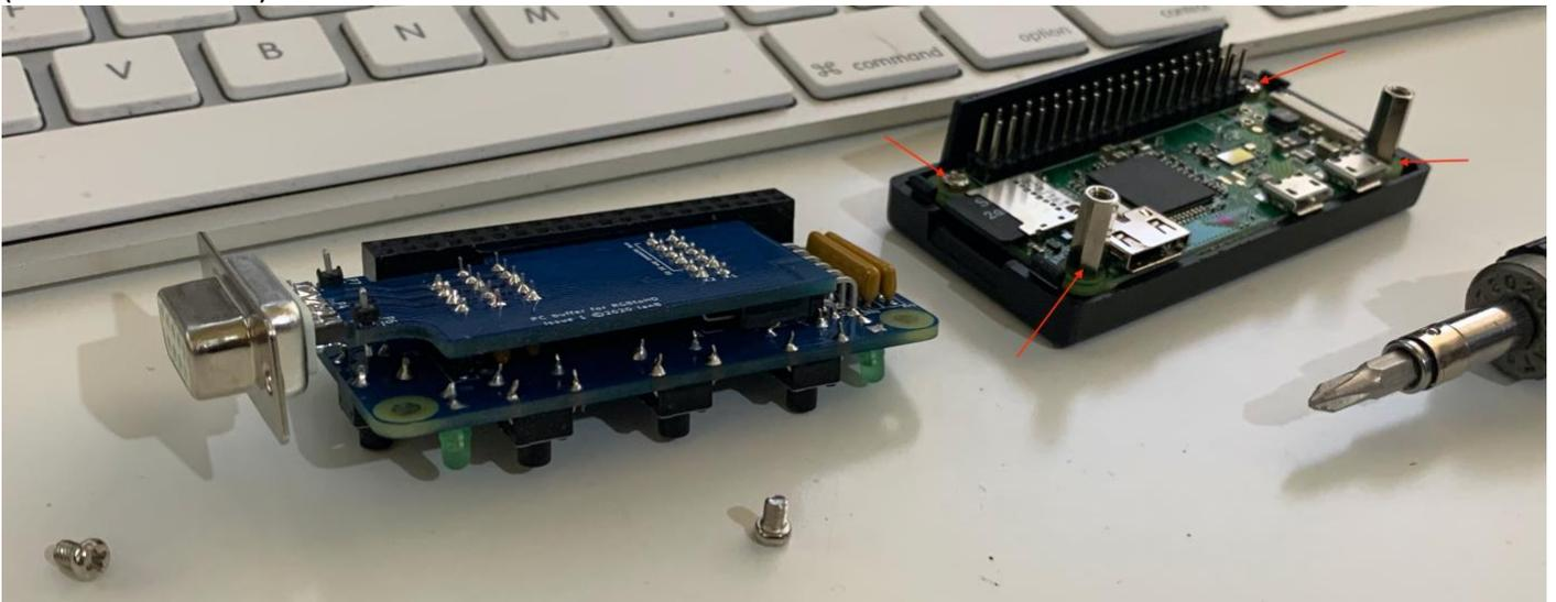
Carefully align and install the RGBtoHDMI sandwich on top of the Pi Zero WH header - then install the remaining 2 screws as shown below.
