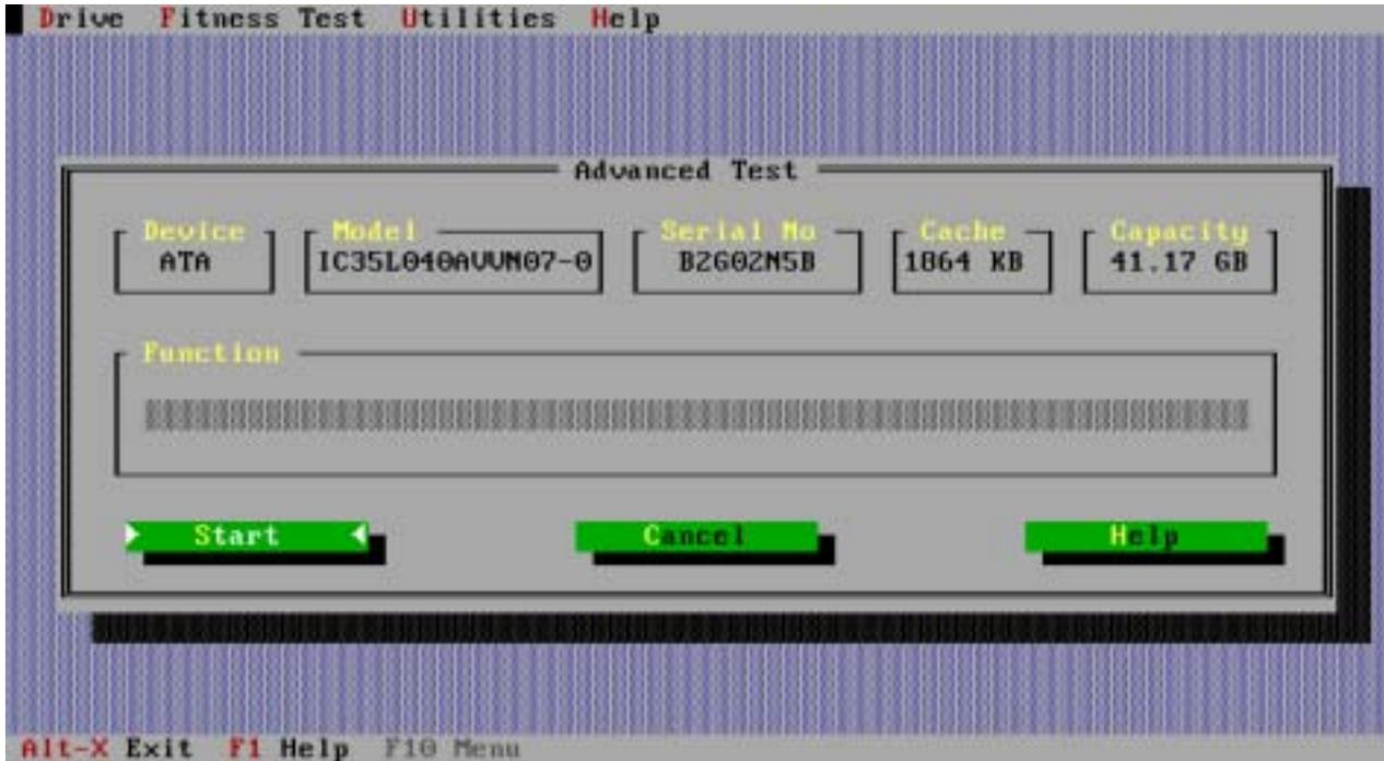
DFT only performs a read test in the user data area, so your data will not be overwritten. Execution time will normally be in the order of 40 minutes, but this can be longer for very large capacity drives. Test progress will be illustrated as shown below.
