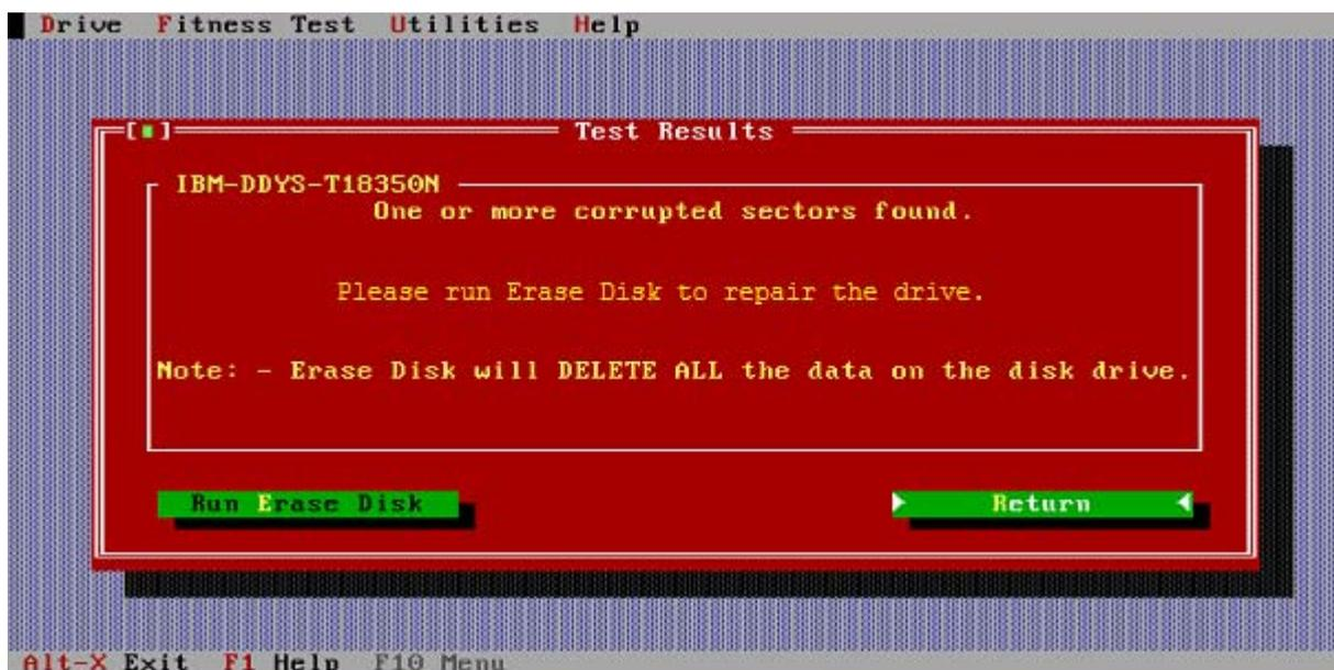
In most cases when DFT reports a media error this is because the data in a sector cannot be read due to corruption. These corrupted sectors can be recovered by being re-written, see options below.
