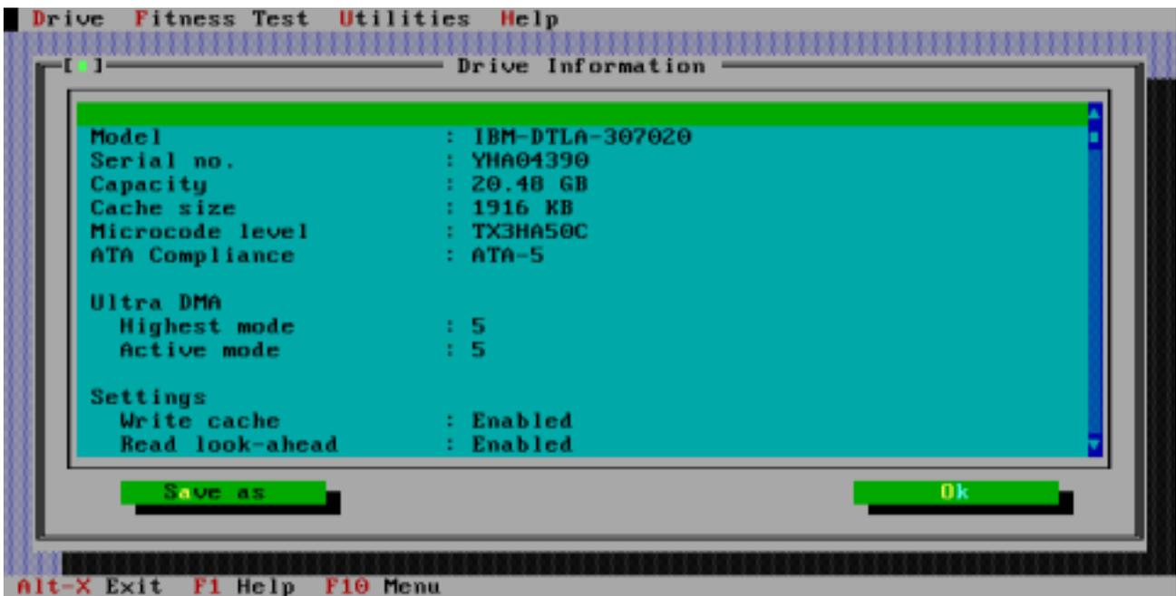
The drive information displayed above can be saved to a text file in the **DATA** sub-directory on the floppy drive. The default name of the text file is **DRVINFO.TXT** as shown below, you can change the filename by over typing this name with, for example, the drive serial number.
