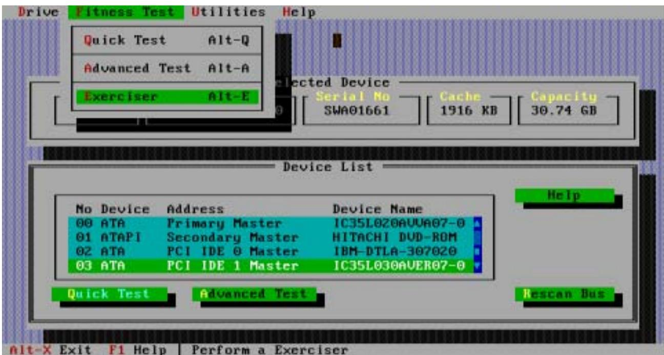
The Exerciser is basically the **Advanced Test** with the addition of a number of 30-minute drive tests. The number of 30-minute periods can be set in the following option screen. The pass / fail / abort mechanism are similar to that of Quick Test.
