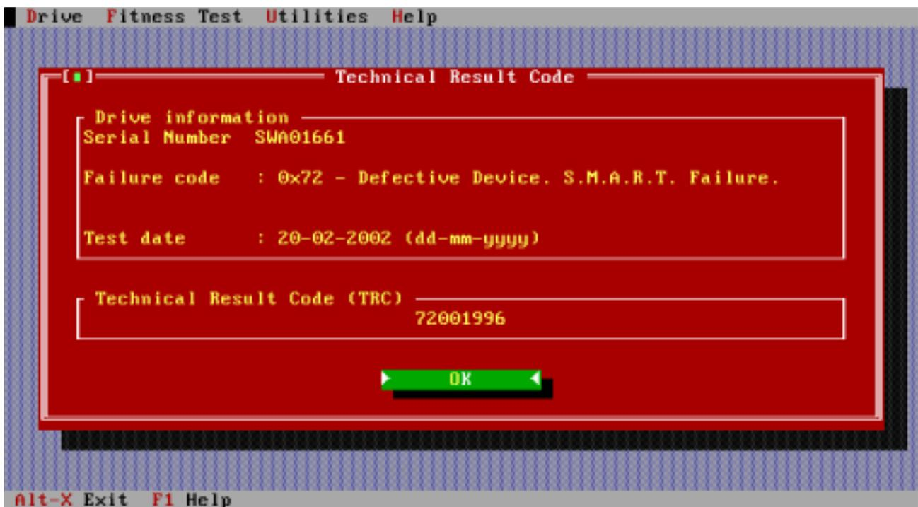
The failing return code 0x72 represents a S.M.A.R.T. error. The S.M.A.R.T. system is a disk drive's way of notifying of possible failure in the future (see Utilities Section of this document for more information on S.M.A.R.T).
