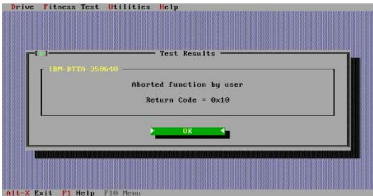
This says that testing has **not** been completed, and is not a statement of either pass or fail. Testing must be restarted and run to completion in order to assess if there is a problem with the drive. The return code 0x10 is not an error.
