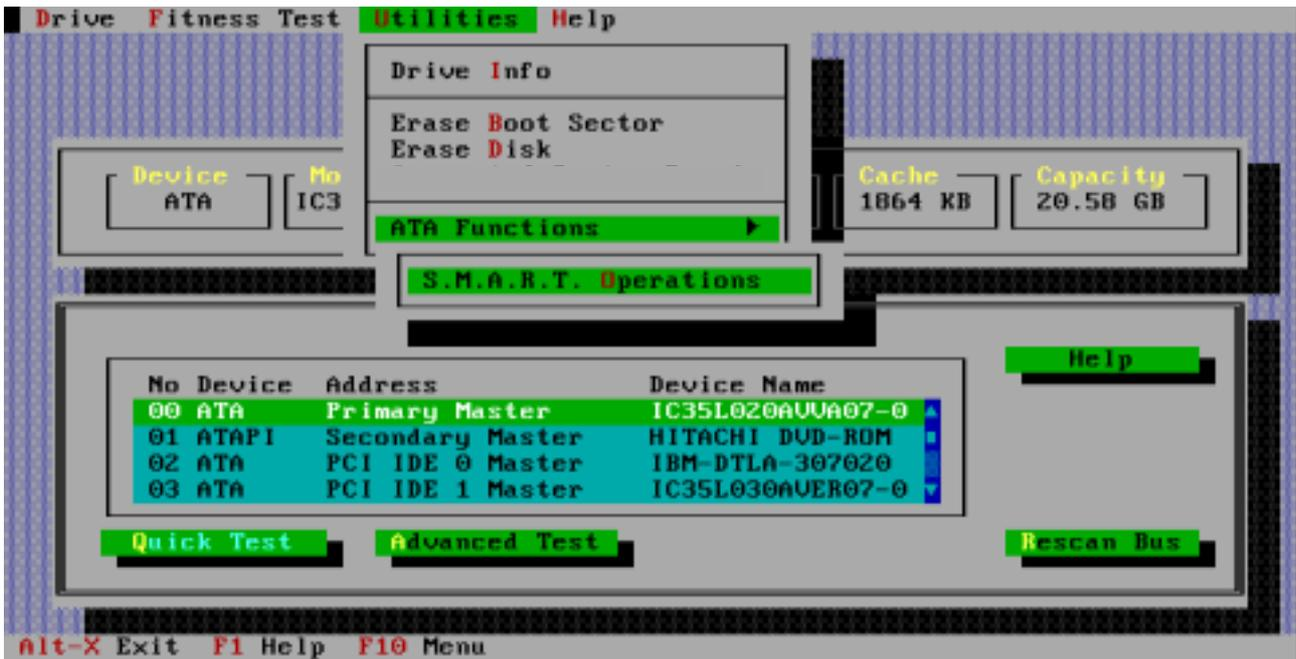
To enable/disable S.M.A.R.T., select S.M.A.R.T. Operations from the utilities menu as shown above, S.M.A.R.T. can now be enabled or disabled on the selected drive by selecting enable/disable as shown below.
