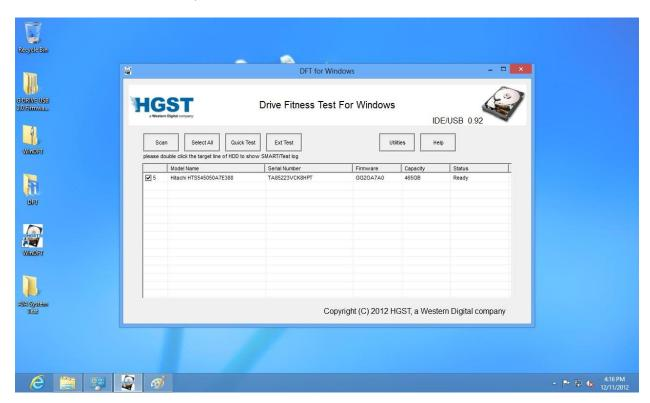
3. Click on Quick Test to run the Quick Test, or Ext Test to run the Extended Test. The Quick test should take a few minutes to run where as the Extended test will take much longer depending on the capacity of your drive.
