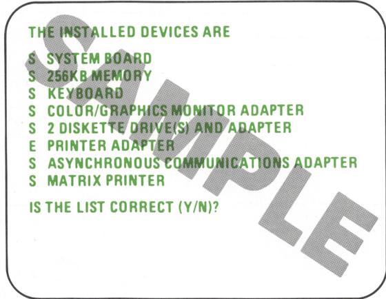
**Note:** The IBM Communications Cable and the Printer Cable will not appear in the list. The Graphics Printer will be listed as "Matrix Printer." The Game Control Adapter may not be listed if the joysticks or paddles are not connected when the Power is set to On.
