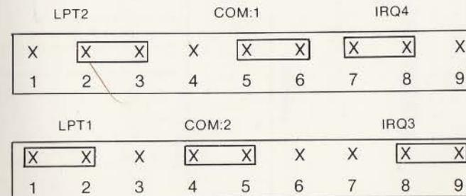
\* To disable the serial or parallel port simply remove the appropriate jumper shunts.
