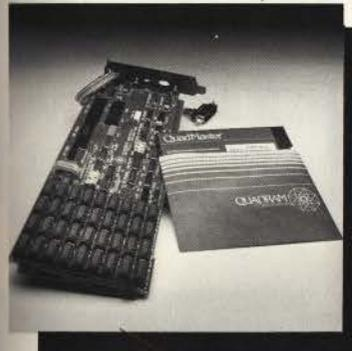
Quadram's Quadboard II is an all-on-one board which combines six IBM PC functions in one. This multifunction board combines two serial ports, chronograph, and memory expansion — all compatible with IBM PC hardware. The two RC-232 async ports can be used for modems, printers, and other serial devices. Memory expansion is socketed and fully expandable in 64K increments up to 256K. Full parity generation and checking are standard. Also included is complete Quadmaster II software.
