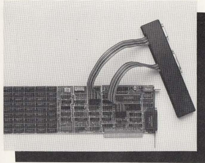
Fig. 6: Quadboard ready for installation
