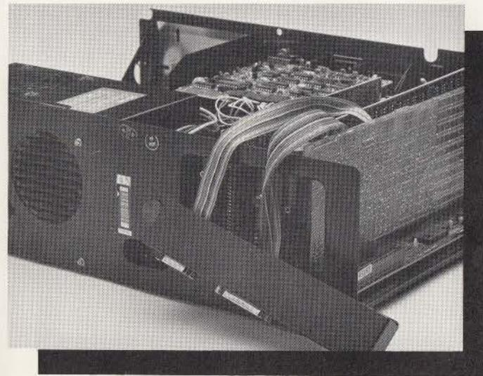
Fig. 7: Quadboard installed and ready for bracket installation
