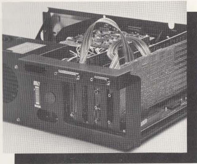
Fig. 8: Attaching the bracket to the PC chassis
