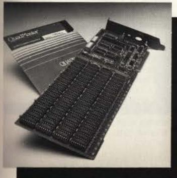
Now IBM PC owners can enjoy faster computing times and more capabilities with the Quad 512+. This board from Quadram combines memory expansion of 512K RAM in increments of 64K, 256K, or 512K with a serial port. The RS-232C async serial port uses the same chip as the IBM serial board and is used for connecting modems, printers, and other serial devices. Also included is complete Quadmaster II software.
