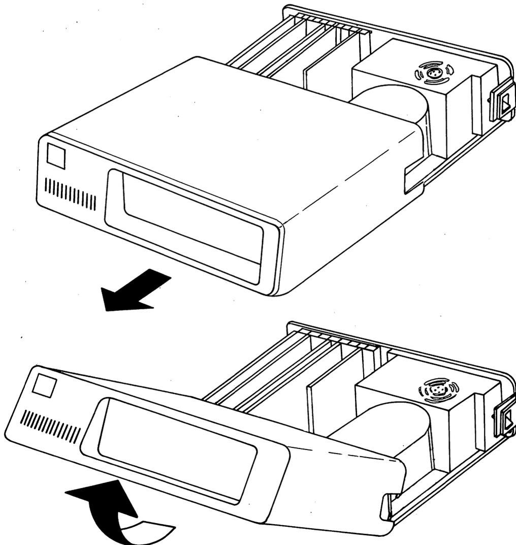
\* If the cover doesn't slide, check for snags between the cover and cables.
