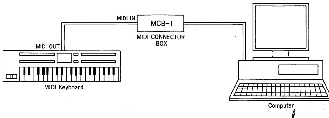
\* The sound source in the LAPC-I can be sounded even without using software, if an external keyboard is used for performance. When software is to be used, set THRU in the MIDI interface section to "ON" by means of the software. When THRU is not ON, performance information originating from the computer will generate sound, but an external keyboard will not produce sound. For details, refer to the manual for the software used.
