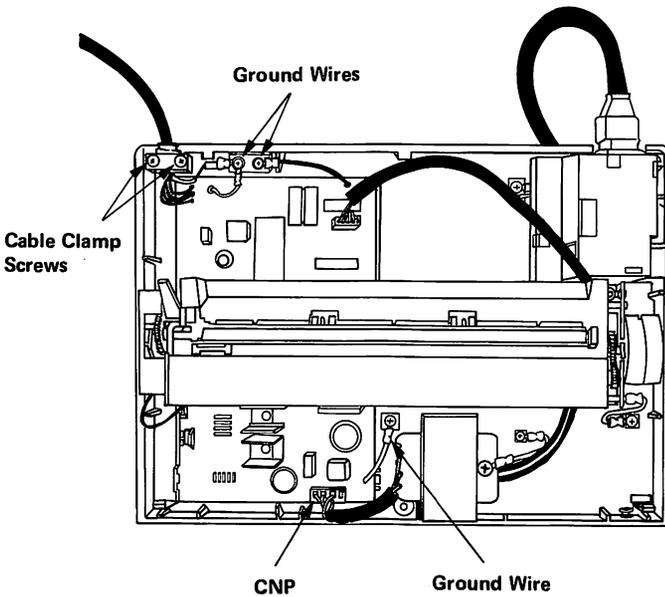
8. Press the three logic card latches away from the logic card, and lift the card out of the bottom cover.
