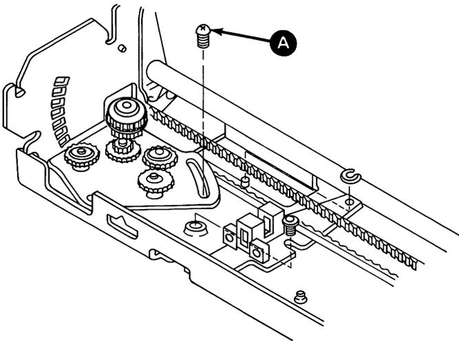
12. Lift belt off pulley at each end.
