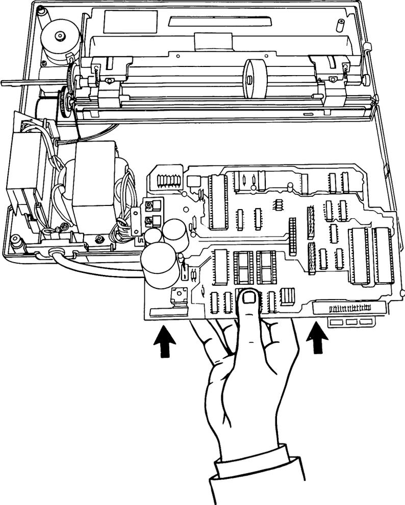
2. Align six holes in control circuit card with six posts in base cover.
