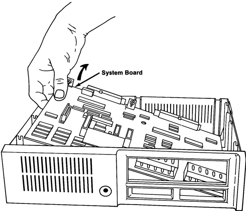
13. Remove the four system board mounting screws
