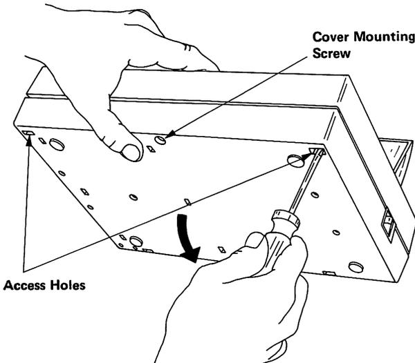
8. Lift the front of the top cover up, and slide it towards the front of the printer to separate it from the bottom cover.
