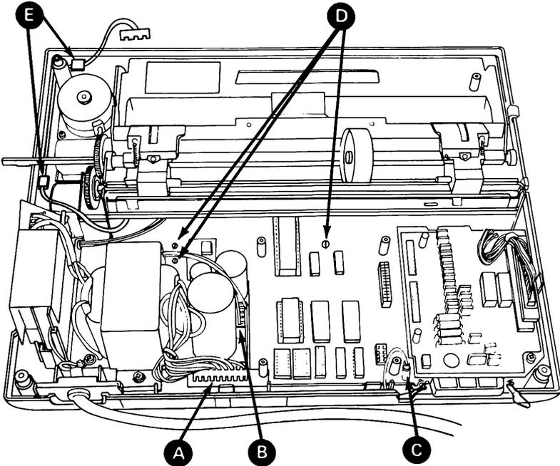
12. Press three tabs **A**, **B**, and **C**. Lift card clear of tabs.
