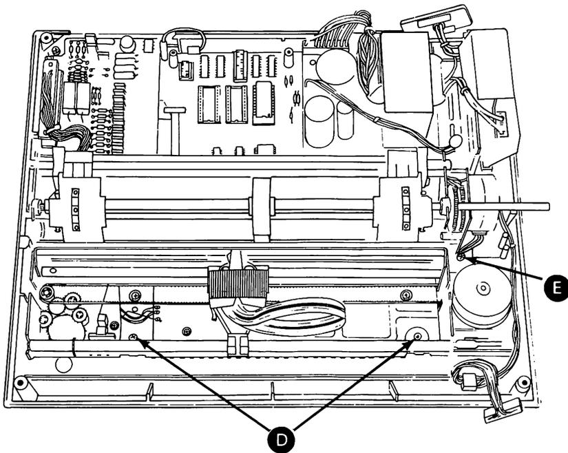
6. Install screw **E** in ground strap.
