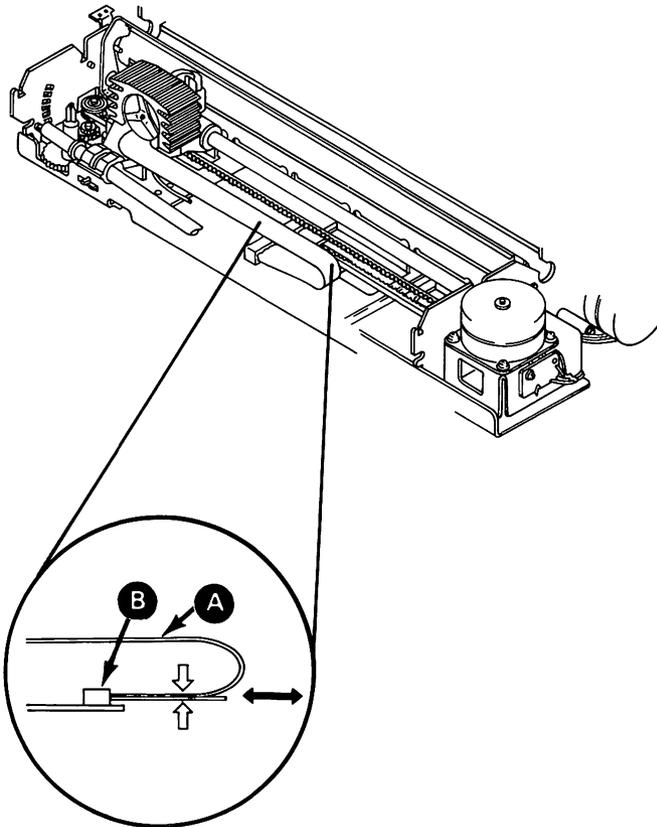
8. Pivot print head lock lever **A** clockwise.
