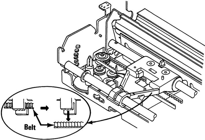
10. Loosen screw in slot in carriage drive assembly **A**.
