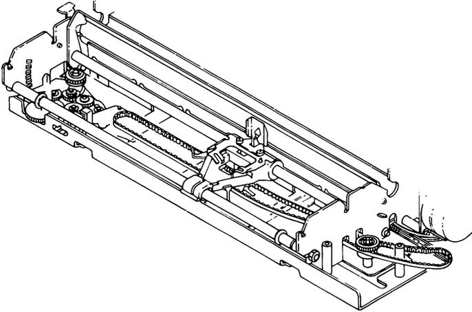
3. Place belt onto pulleys at both ends.
