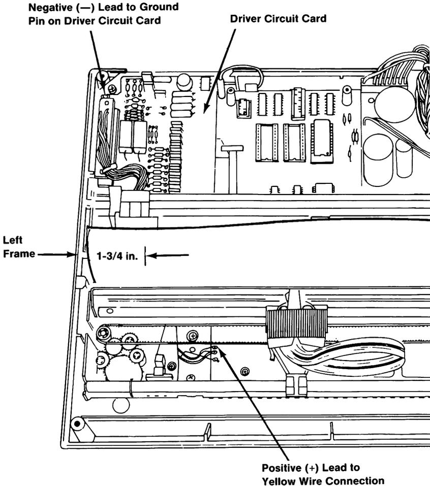
15. Move the left margin sensor to the left until the voltage reading on the meter is a down level (approximately 0 Vdc).
