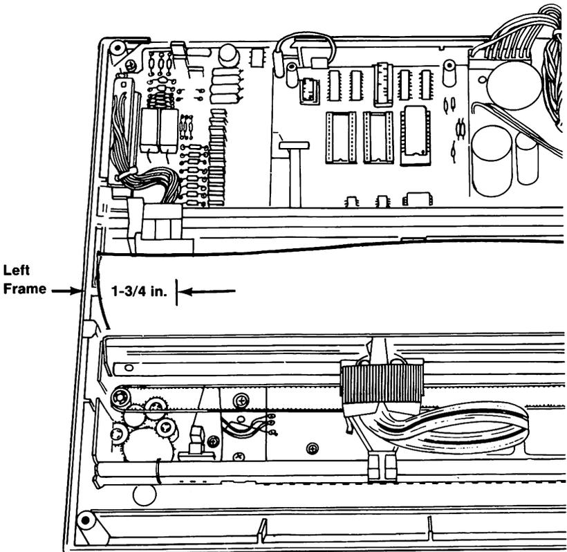
9. Loosen the left margin sensor locking screw.
