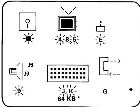
The IDs for joystick and sound always blink because their interfaces are on the system board. The blinking does NOT mean a joystick or external speaker is installed.
