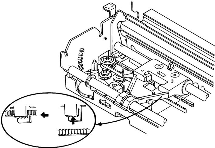
5. Place carriage motor onto motor mounts **A**.
