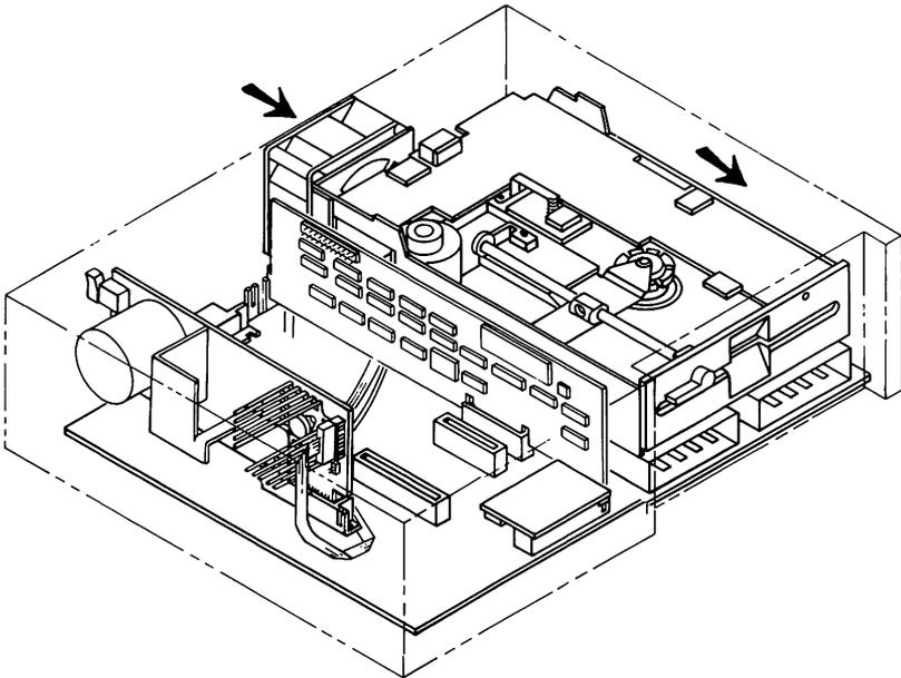
8. Two studs hold the rear of the diskette drive to the system board. Pull up on the rear of the diskette-drive mounting bracket until the studs are clear of the system board. **DO NOT PULL ON THE CIRCUIT BOARD.**
