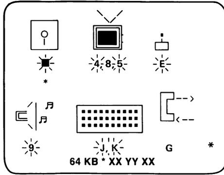
If something other than “\*” appears, a failure was detected and you should follow the PIC for that test.
