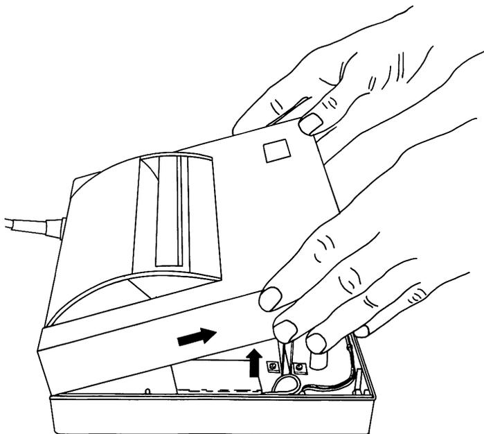
9. When the covers are separated, set the top cover off to the side and disconnect CNK (control panel cable) from the logic card.
