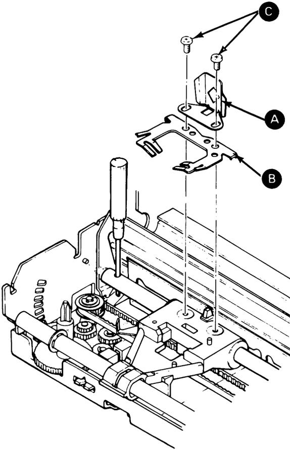
3. Position shield and plate as shown. Tighten screws.
