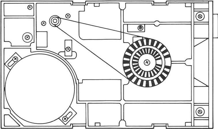
**IS THE DRIVE BELT INSTALLED ON THE PULLEYS AND IN GOOD CONDITION?**
