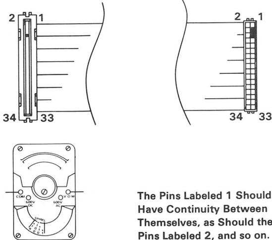
The Pins Labeled 1 Should Have Continuity Between Themselves, as Should the Pins Labeled 2, and so on.
