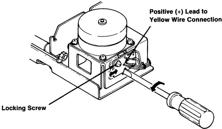
21. Move the print head slightly to the left. The voltage reading should drop to a down level (approximately 0 Vdc). Do not allow the print head to step to the next detented position.
