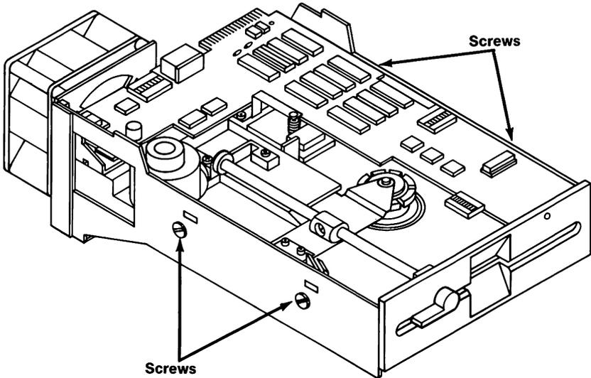
5. Push the diskette drive to the front, so that the diskette drive slides forward in the mounting bracket and rests against the opening in the front of the system unit.
