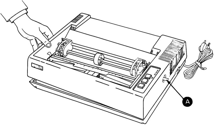
2. Connect control panel cable to control panel.
