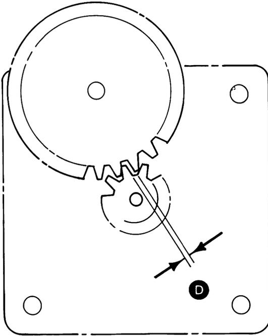
13. Tighten motor mounts screws.
