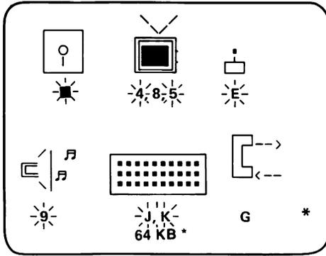
The advanced-test menu consists of symbols, with each symbol representing one area of the IBM PCjr. The letters or numbers below the symbols are IDs of tests you can perform. A quick way to determine if you are looking at the advanced-test menu or the customer-level test menu (they look similar) is to observe the ID under the joystick symbol. The advanced-test level has an “E” there. The customer-level has a “6.”
