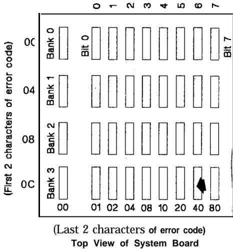
Figure 4-10. System Board (Top View)
