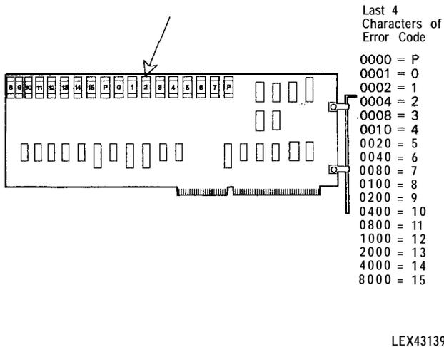
Figure 9-24. Failing Module Location
