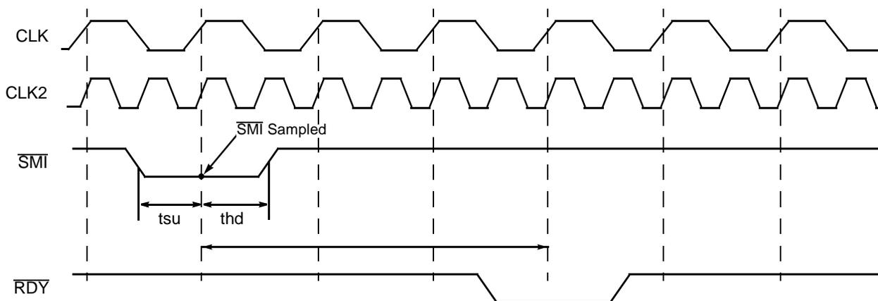
Figure 24. SMI Timing for Servicing an I/O Trap
