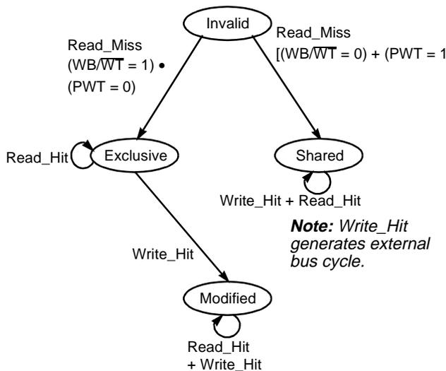
**Figure 1. Processor-Induced Line Transitions in Write-Back Mode**
