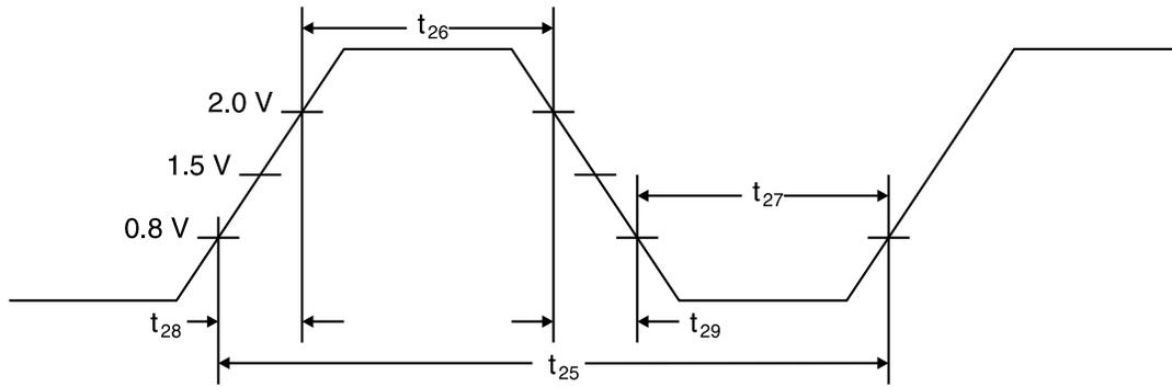
Figure 45. TCK Waveforms
