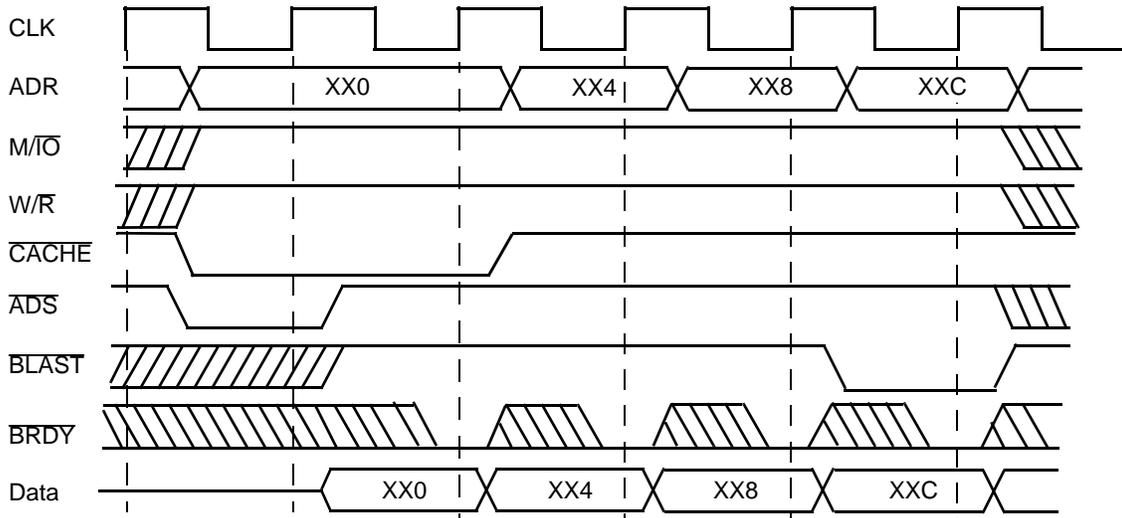
Figure 16. Burst Write
