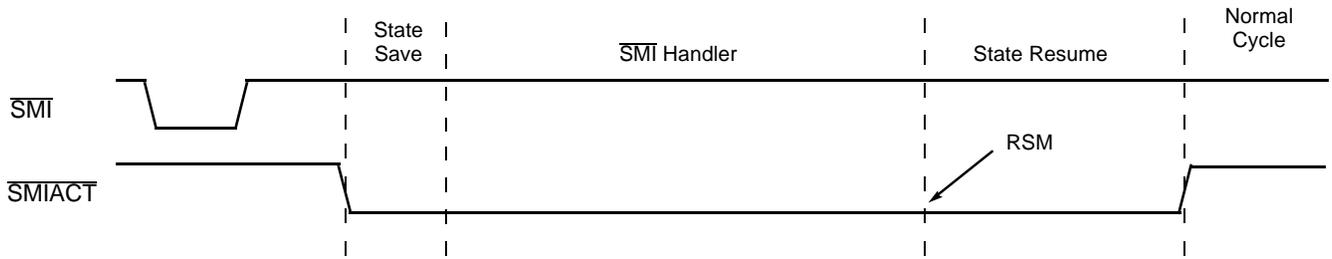
**Figure 33. SMM Timing in Systems Using Non-Overlaid Memory Space and Write-Through Mode with Caching Enabled During SMM**
