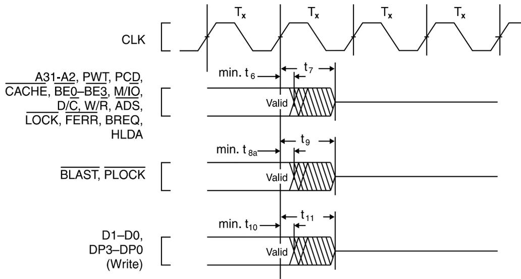
Figure 41. Maximum Float Delay Timing
