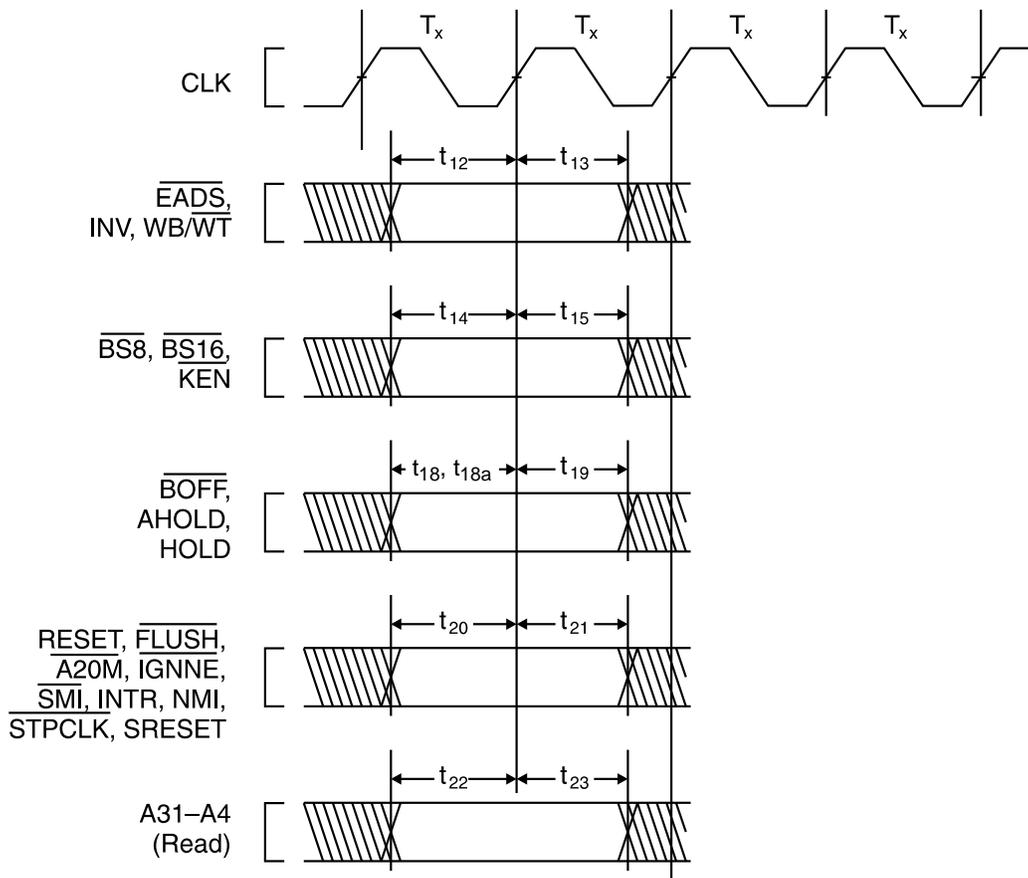
Figure 43. Input Setup and Hold Timing
