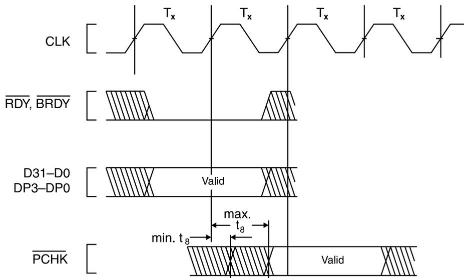
Figure 42.  $\overline{PCHK}$  Valid Delay Timing
