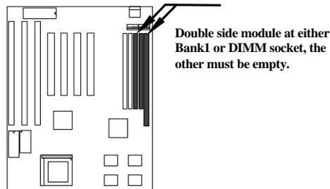
Following table explains more about the RAS limitation. You can see that Bank1 1st side and DIMM 2nd side use the same RAS3#, and Bank1 2nd side and DIMM 1st side use the same RAS4#. If you are using single side SIMM at Bank1 and single side DIMM, it should be no problem. But if you are using double side DIMM or double side SIMM at Bank1, the other must be empty.
