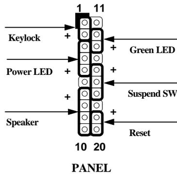
Other housings may have a 12-pin connector. If your housing has this type of connector, connect it to PANEL as shown in the figure. Make sure that the red wire of the connector is attached to +5V.
