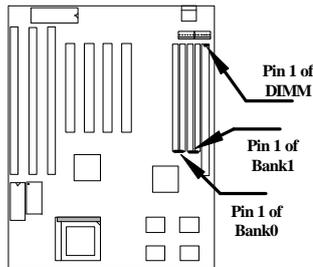
This mainboard has four 72 pin SIMM sockets (Single-in-line Memory Module) and one 168 pin DIMM socket (Dual-in-line Memory Module) that allow you to install system memory from minimum 8MB up to maximum 128MB.
