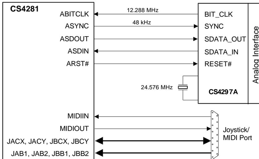
**Figure 9. Single AC '97 Codec Connection Diagram**
