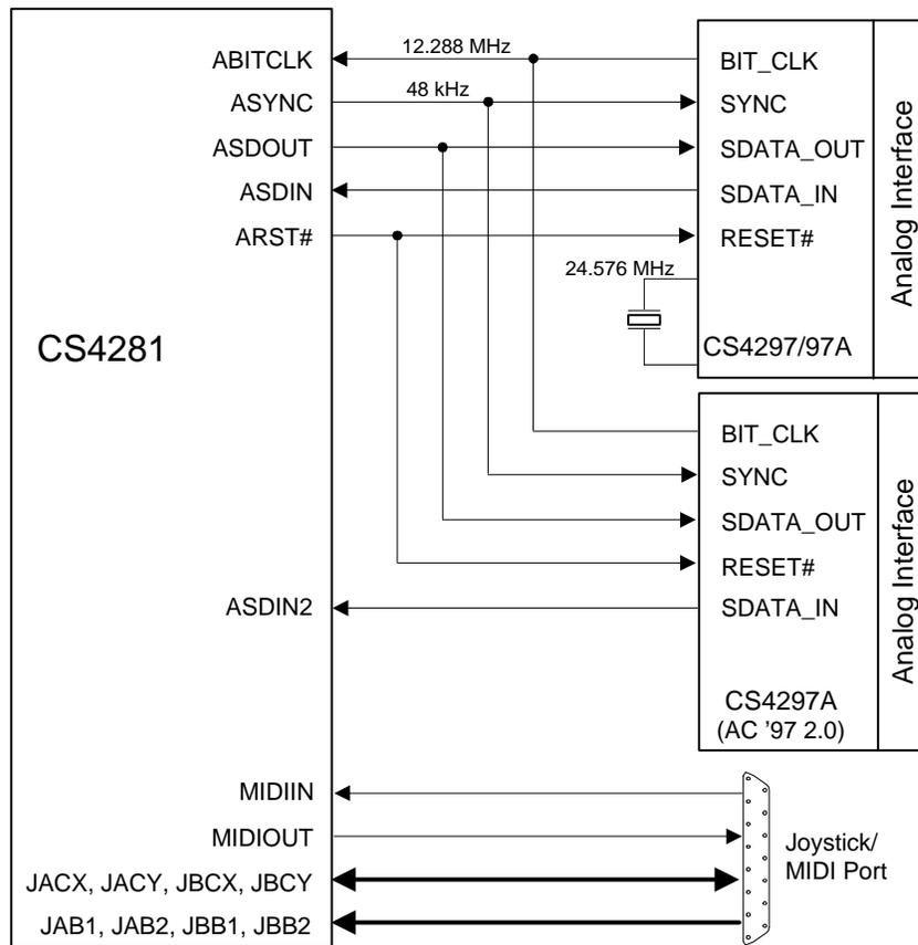
**Figure 10. Dual AC '97 Codec Connection Diagram**
