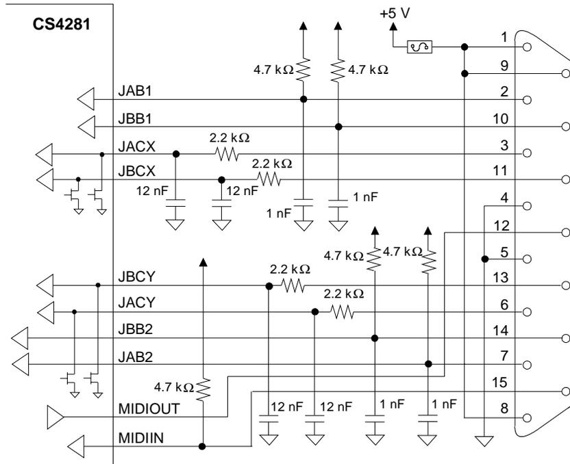
**Figure 12. Joystick Logic**
