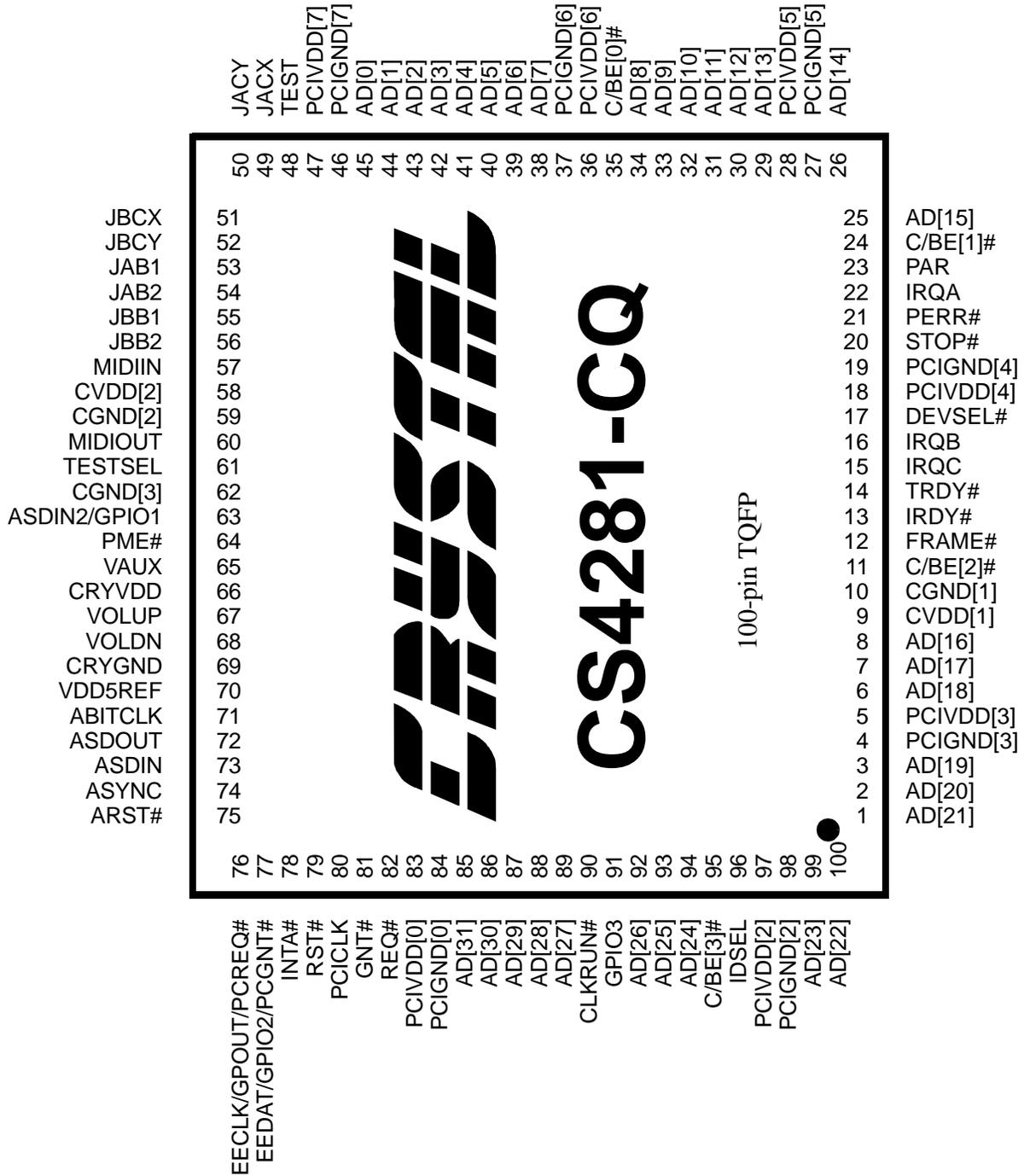
A '#' sign suffix on a pin names indicates an active-low signal.
