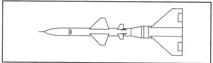
Figure 5-1: The SA-2 "Guideline" is a prime example of a beam-riding surface-to-air missile.
