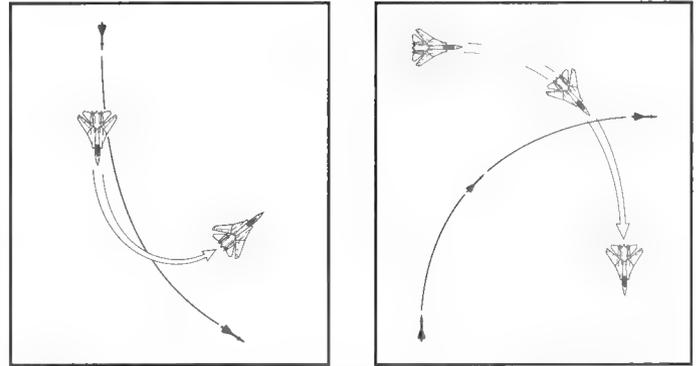
Figure 5-7: These diagrams show how playing the angles can defeat the tracking solution of an in-coming missile.
