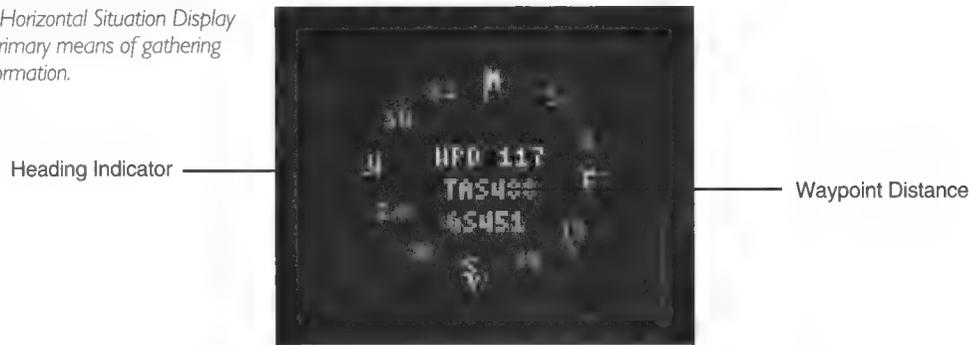
The Horizontal Situation Display (HSD) consists of a rotating compass dial with three lines of navigational text inserted in the center. Like the VDI, it is multi-functional. This monitor can alternate between showing standard HSD navigational information and being a Target Information Display (TID) repeater.
