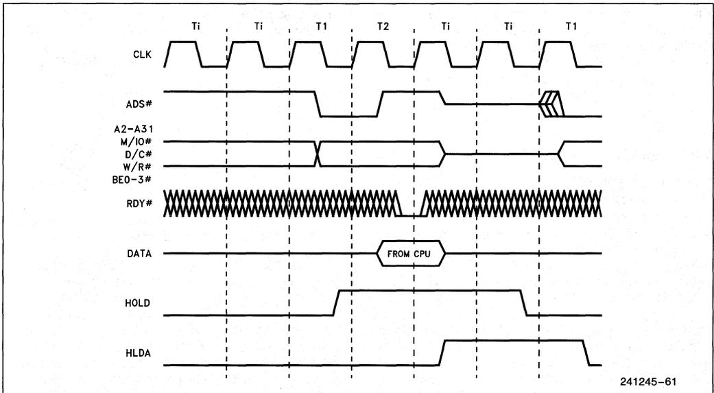
Figure 7.26. HOLD/HLDA Cycles
