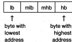
The function of unaligned transfers with dynamic bus sizing is not obvious. When the external systems asserts BS16# or BS8# forcing extra cycles, low-order bytes or words are transferred first (opposite to the example above). When the Intel486 DX microprocessor requests a 4-byte read and the external system asserts BS16#, the lower 2 bytes are read first followed by the upper 2 bytes.
