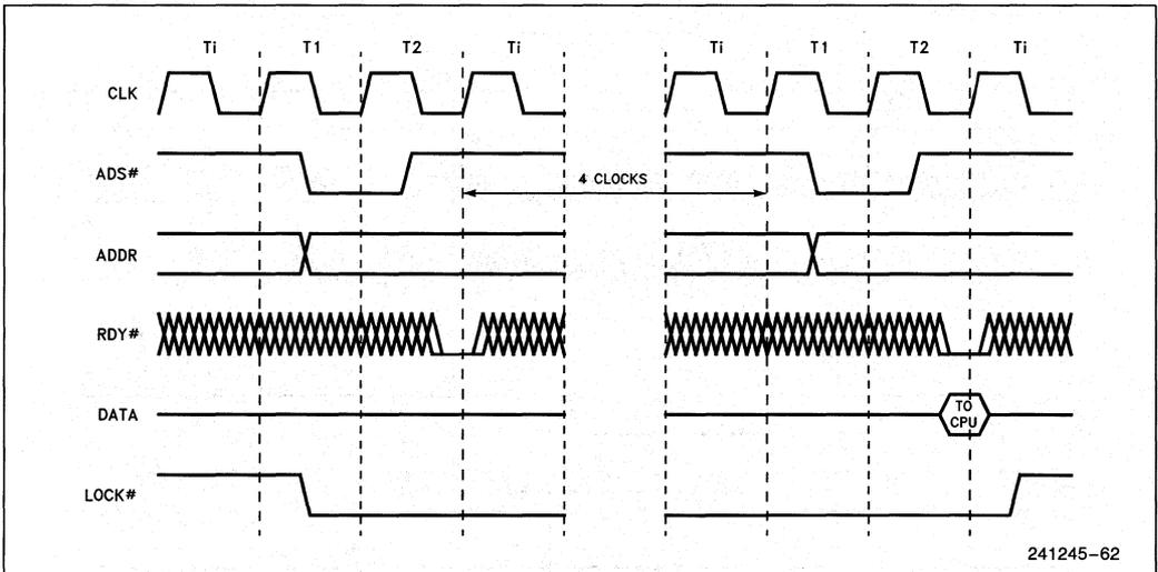
Figure 7.27. Interrupt Acknowledge Cycles
