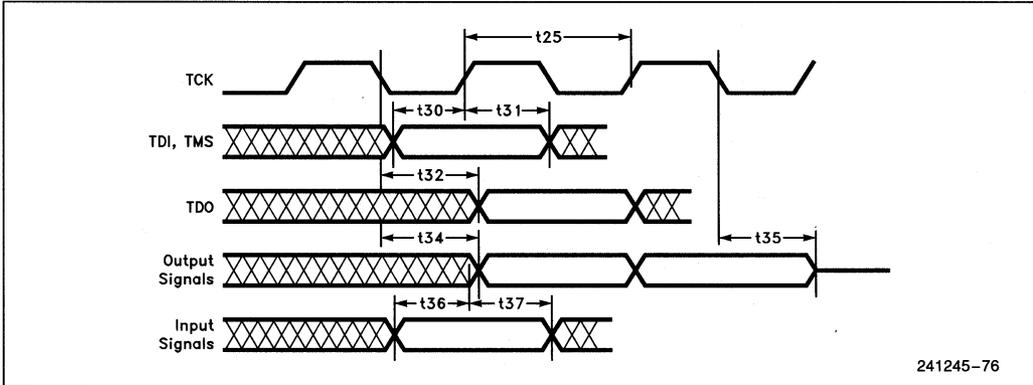
Figure 14.7. Test Signal Timing Diagram
