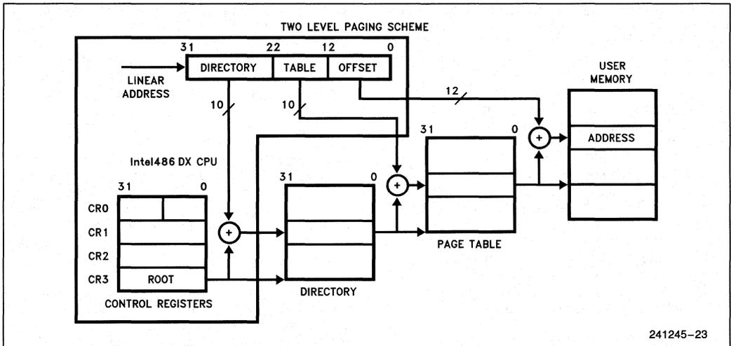
**Figure 4.19. Paging Mechanism**
