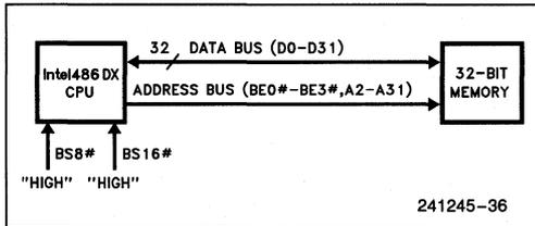
Figure 7.3. Intel486™ DX Microprocessor with 32-Bit Memory
