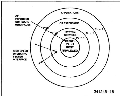
Figure 4.14. Four-Level Hierarchical Protection
