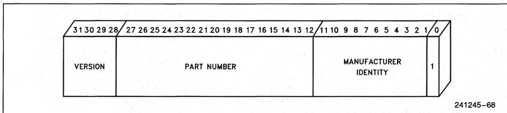
**Figure 8.2. Format of Device Identification Register**
