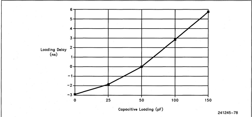
**14.4.3.b TYPICAL LOADING DELAY VERSUS CAPACITIVE LOADING UNDER WORST-CASE CONDITIONS FOR A LOW TO HIGH TRANSITION ON THE INTEL486 DX2 CPU**
