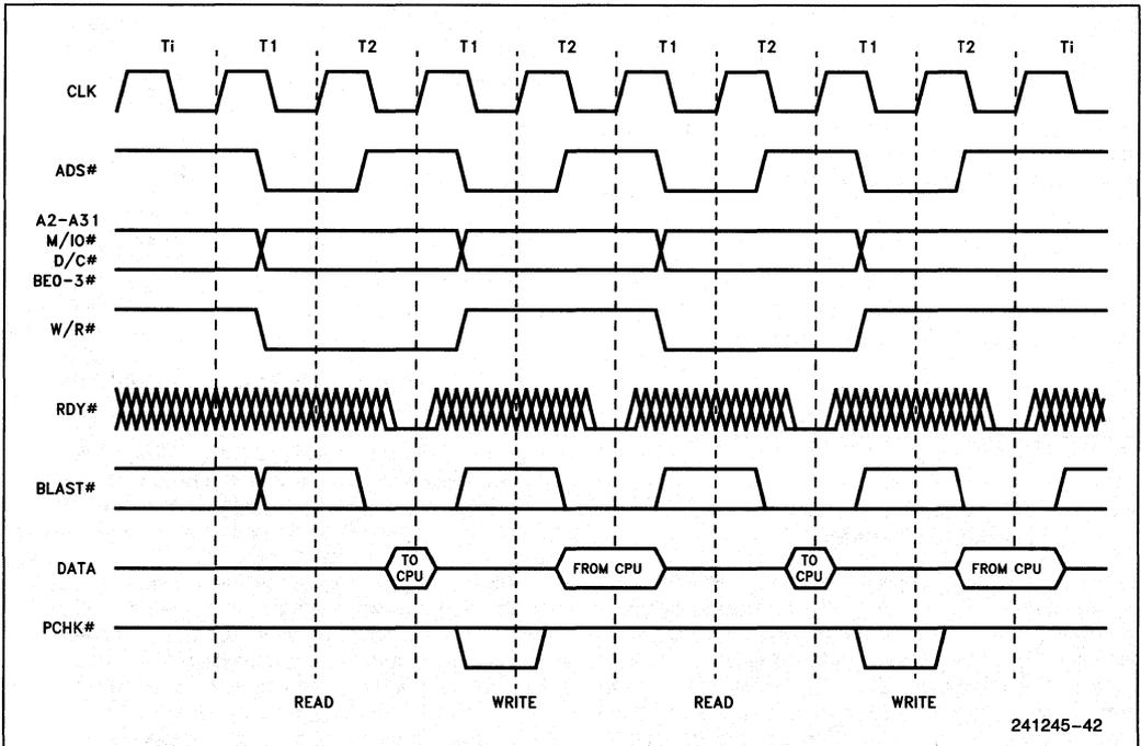
Figure 7.7. Basic 2-2 Bus Cycle
