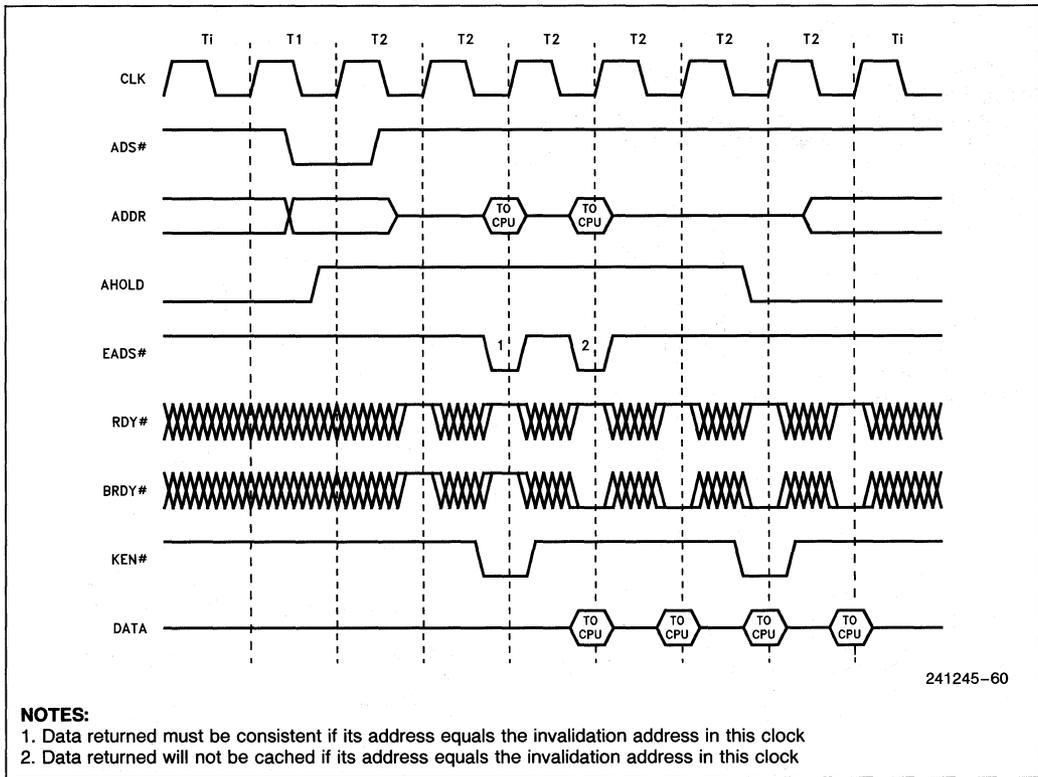
**Figure 7.25. Cache Invalidation Cycle Concurrent with Line Fill**
