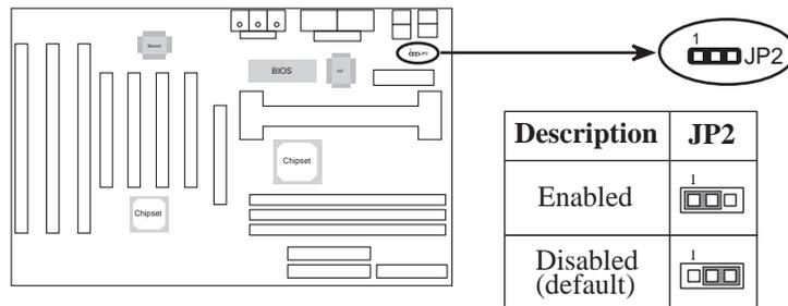
*Note: Make sure that the system power can provide 720mA on +5VSB(+5V Standby) signal before using Keyboard Power On function.*
