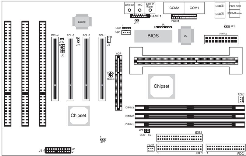
Figure 2-1. Mainboard Component Locations
