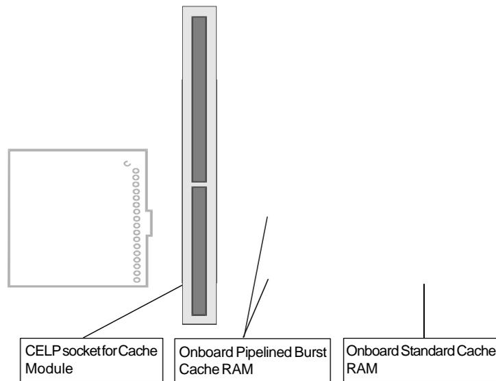
541 mainboard support several types cache scheme including onboard standard asynchronous cache RAM, standard asynchronous cache module, onboard pipelined burst cache SRAM, and pipelined burst cache module.
