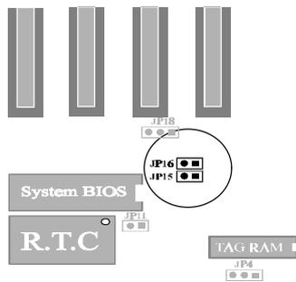
541 mainboard features a clock generator to provide adjustable system clock frequency. JP15 and JP16 are 2-pin jumpers which determine the system clock frequency.
