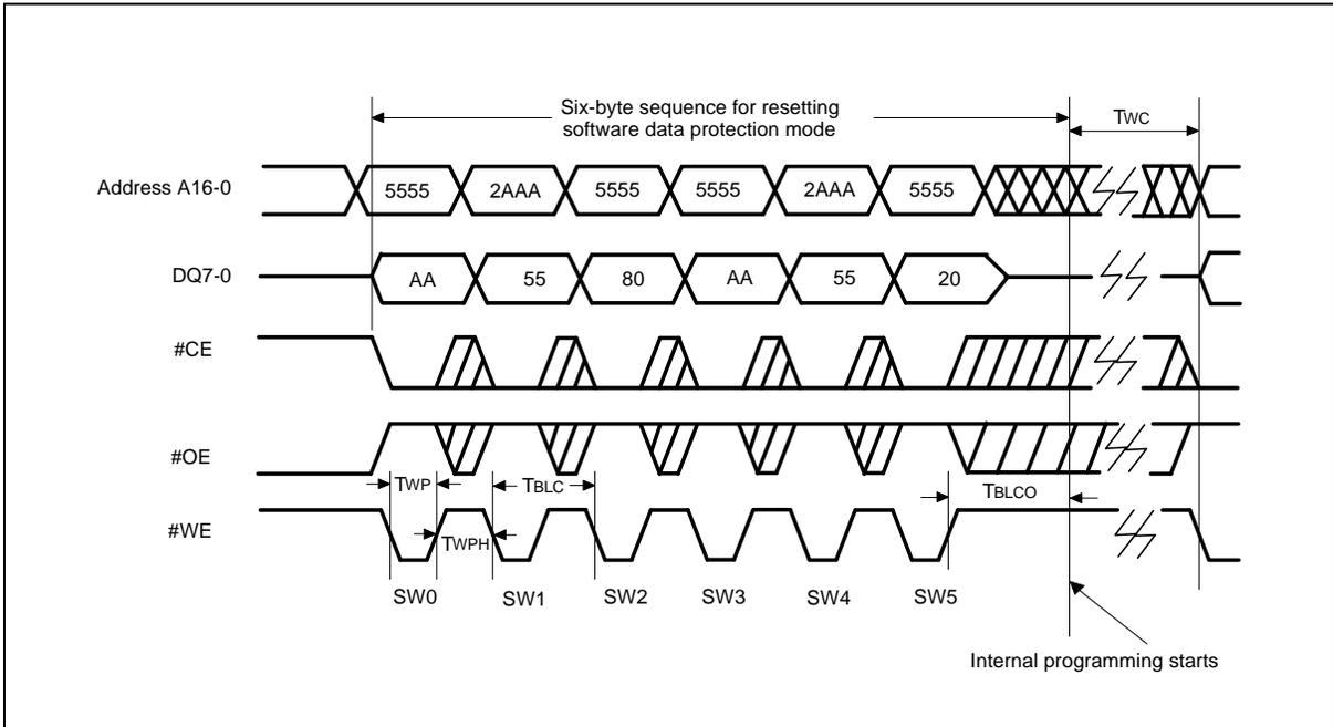
**5 Volt-only Software Chip Erase Timing Diagram**
