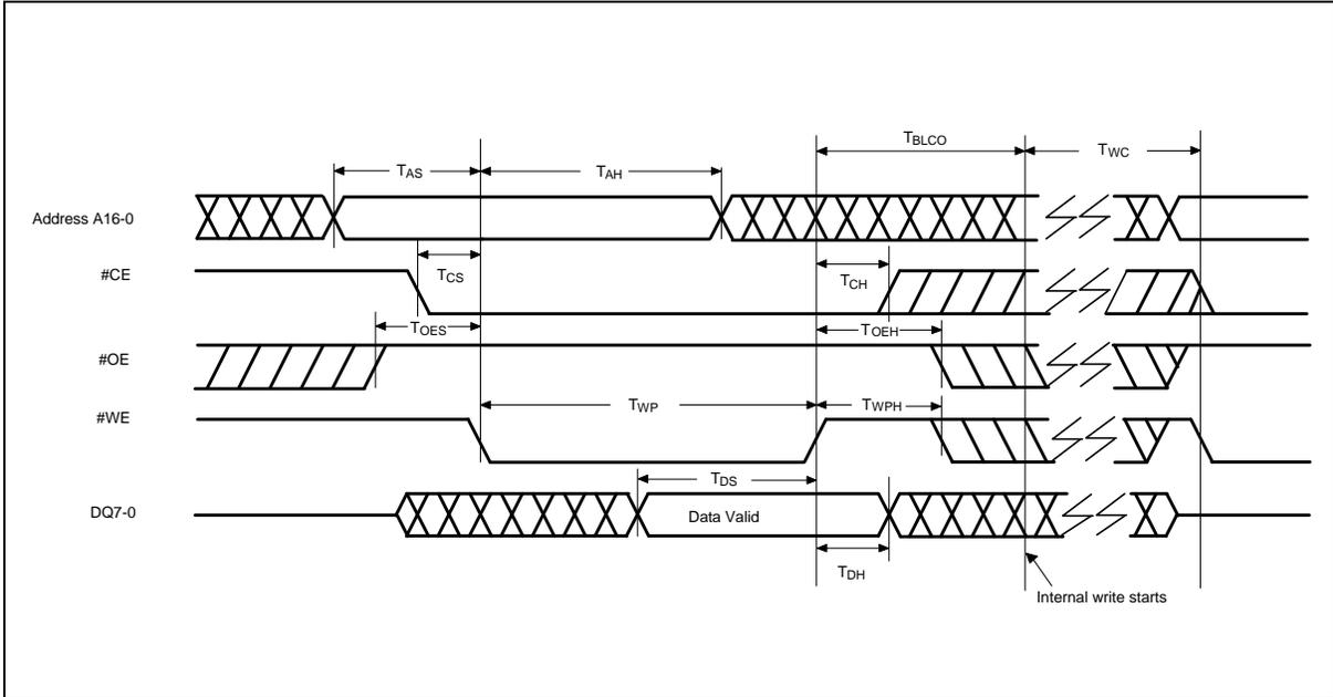
**#CE Controlled Write Cycle Timing Diagram**
