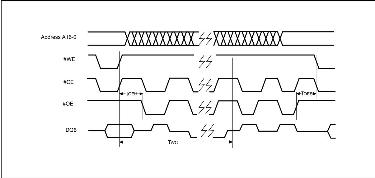
**Page Write Timing Diagram Software Data Protection Mode**
