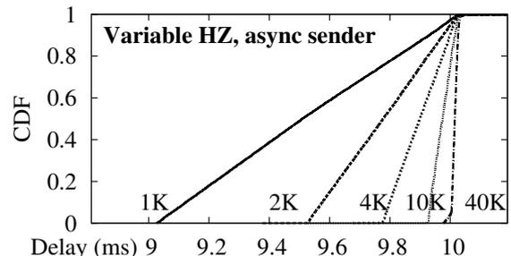
Figure 6: Distribution of delays for a 10ms pipe and different HZ values, asynchronous senders.
