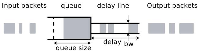
Figure 2: The structure of a dummynet “pipe”. Configurable parameters include bandwidth, delay and queue size.
