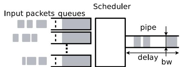
Figure 4: The binding between queues, scheduling algorithm and the corresponding pipe.
