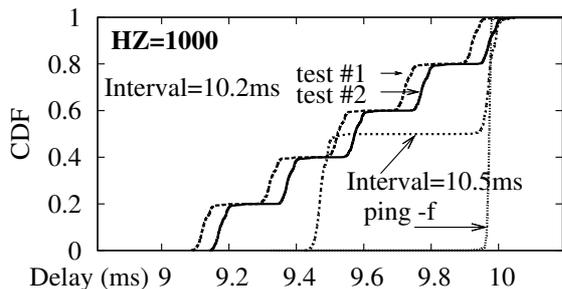
Figure 7: Distribution of delays for a 10ms pipe, HZ=1000, synchronous senders.
