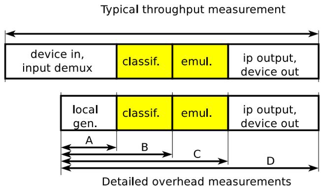
Figure 8: Measurements to determine the emulator's overhead. Top: typical components in PPS measurements. Below: our detailed measurements, to extract the cost of classification and emulation.
