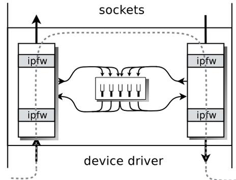
Figure 3: Classifier rules send packets to specific pipes. On exit, the traffic is reinjected into the network stack.
