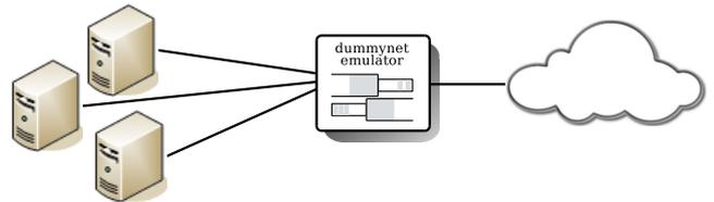
Figure 1: A Dummysnet-enabled bridge can be inserted in an existing the network without any change in the configuration.
