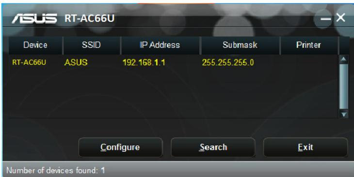
**NOTE:** When you set the router to Access Point mode, you need to use Device Discovery to get the router's IP address.
