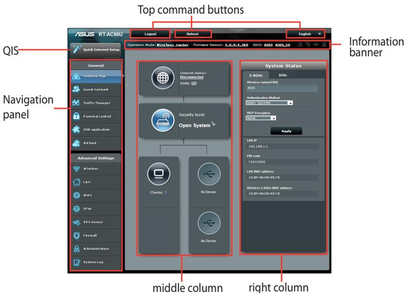
**NOTE:** If you are logging into the Web GUI for the first time, you will be directed to the Quick Internet Setup (QIS) page automatically.
