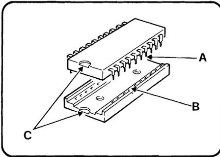
Figure 10 Chip Insertion
