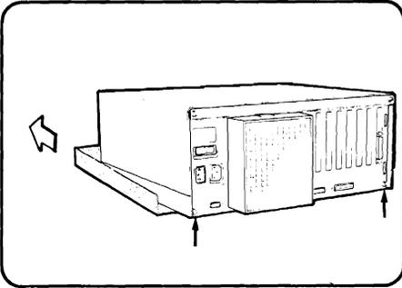
Figure 1 Removal of System Module's Cover
