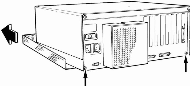
Figure 1 Removal of Basic Module's Cover.
