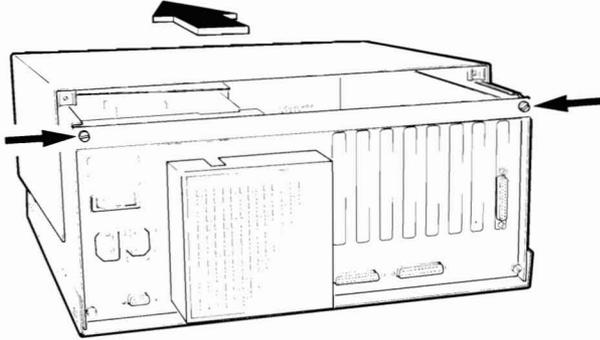
Figure 11 Removal of Basic Module's Covers.
