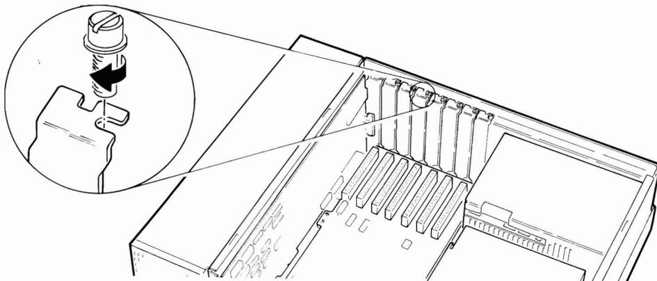
Figure 16 Hole Alignment.
