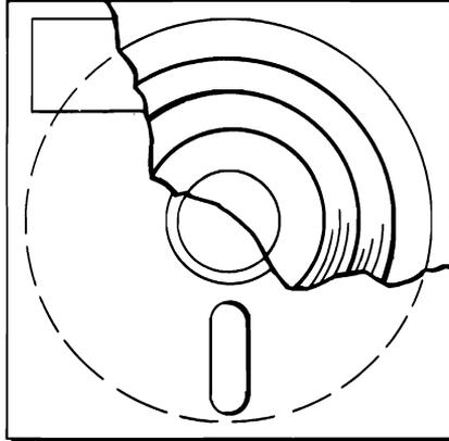
Information is read from or written onto the diskette through the slot in its jacket. When the computer writes information onto the diskette, it does so in unused space. You can also instruct the computer to write over information that is already on a diskette. You might do this to update an inventory file for instance. Note however, if you write new information over old information, the old information is erased – you cannot get it back.
