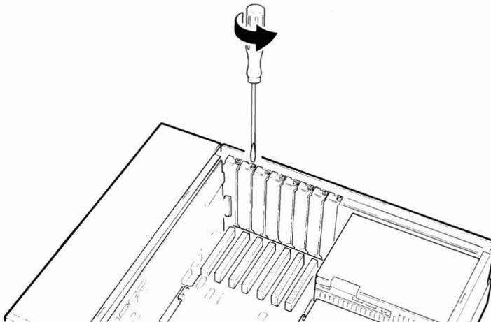
Figure 14 Removal of System Expansion Slot Cover.
