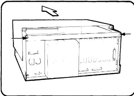
Figure 11 Removal of System Module's Covers
