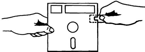
If you want to remove the write-protection, to add or change some information on the diskette, just peel off the write-protect sticker. With the sticker off, the computer can write on the diskette.
