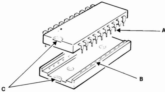
Figure 5 Chip Insertion.
