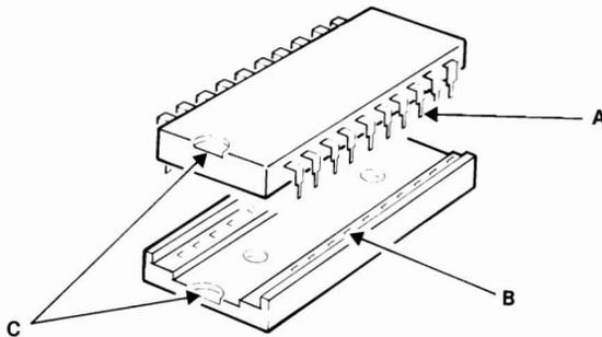
Figure 10 Chip Insertion.
