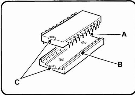
Figure 5 Chip Insertion
