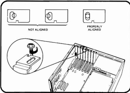
Figure 16 Hole Alignment
