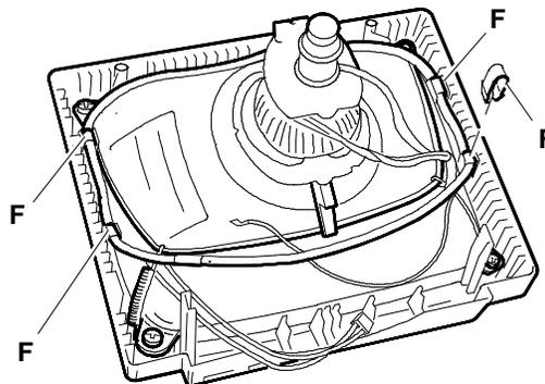
Fig. 3-13 Degaussing coil securing clips removal
