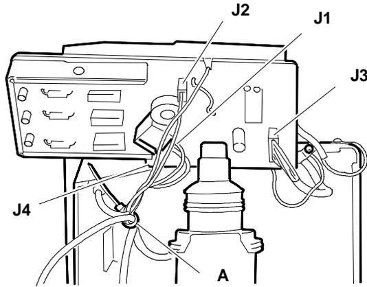
Fig. 3-7 - Position of cable clamp A
