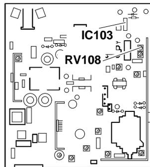
Fig. 3-17 - Frequency adjustment
