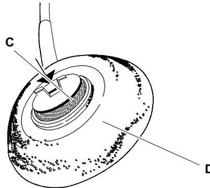
Fig. 3-12 Correct CRT anode fixing
