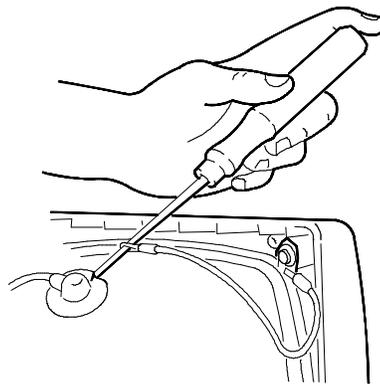
Fig. 3-3 Screwdriver to ground connection
