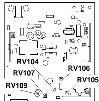
Fig. 3-19 - Vertical linearity adjustment
