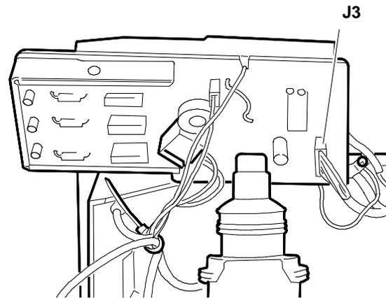
Fig. 3-5 Position of connector J3 on video amplifier board
