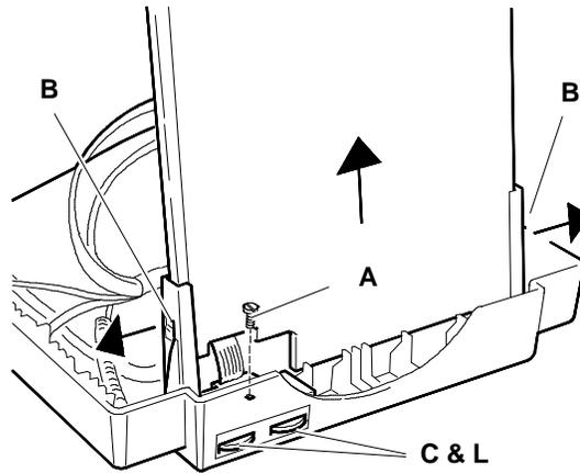
Fig. 3-11 Motherboard removal from video frame
