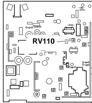
Fig. 3-20 - Distortion (pincushion) adjustment
