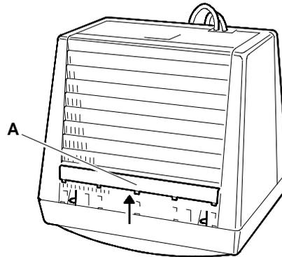
Fig. 3-1 Removal of video casing screws plastic covering
