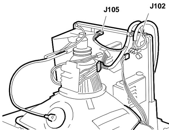
Fig. 3-6 Position of connectors J105 and J102 on the motherboard
