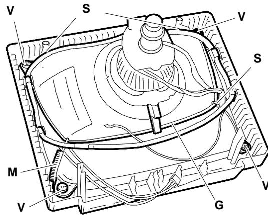
Fig. 3-14 - Position screws securing CRT to video frame
