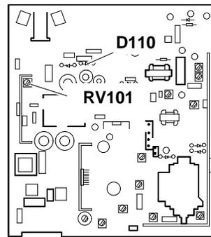
Fig. 3-16 - Voltage adjustment
