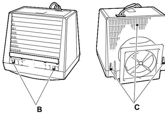
Fig. 3-2 Removal of video casing 5 fixing screws
