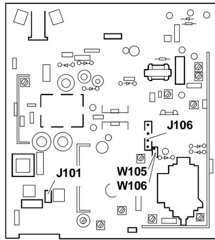
Fig. 3-10 Connector position for connections J101, J106, W105 and W106
