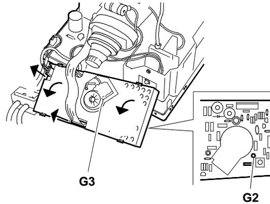
Fig. 4-9 G3 and G2 disconnection from video amplifier board
