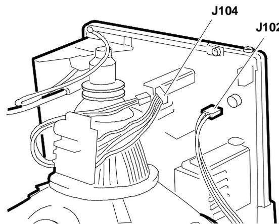
Fig. 4-11 Disconnection of cable from motherboard
