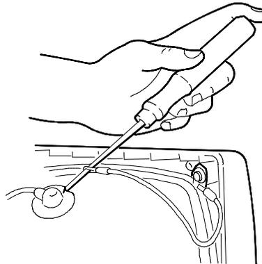
Fig. 4-3 Screwdriver to ground connection
