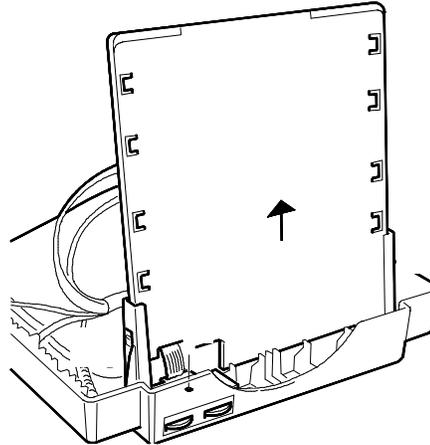
Fig. 4-13 Motherboard solder side metal protection panel removal
