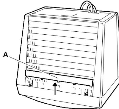
Fig. 4-1 Removal of video casing screws plastic covering
