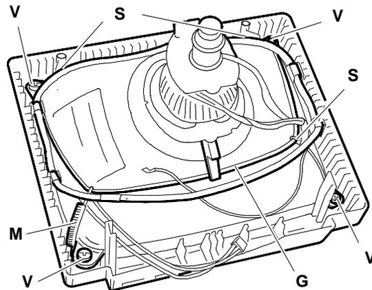
Fig. 4-16 - Position of screws fixing CRT to video frame
