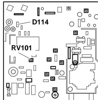
Fig. 4-18 Voltage adjustment
