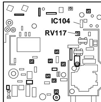
Fig. 4-19 Frequency adjustment
