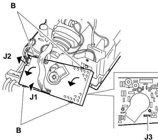
Fig. 4-8 Video amplifier board cables disconnection
