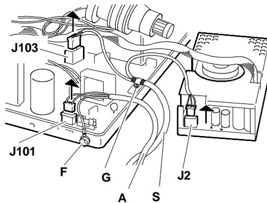
Fig. 4-6 Removal of video signal cable (S) and power cable (A)
