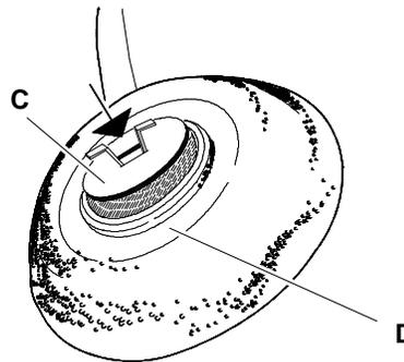
Fig. 4-14 CRT anode correct mounting
