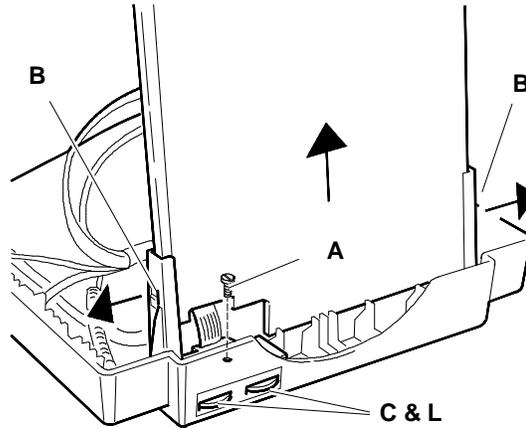
Fig. 4-12 Motherboard structure removal from video casing
