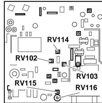
Fig. 4-21 - Vertical linearity adjustment
