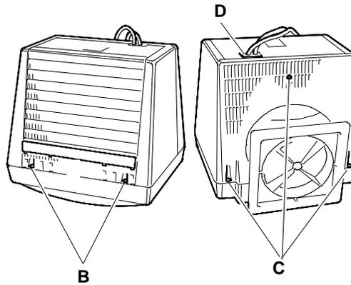
Fig. 4-2 Removal of video casing 6 fixing screws
