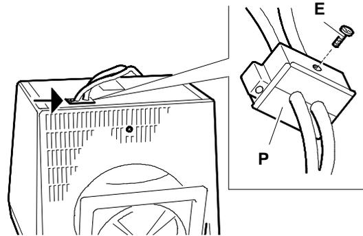
Fig. 4-5 Cable support (P) removal
