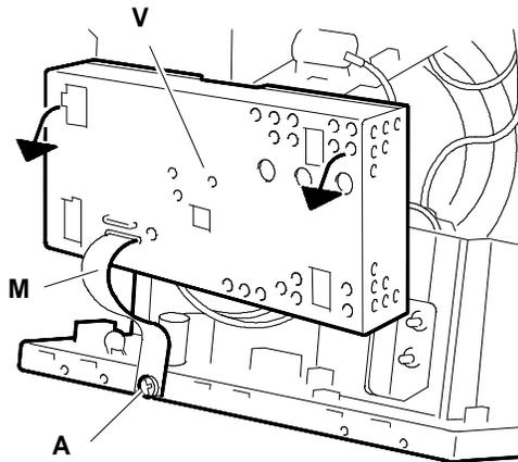
Fig. 4-7 Earthing bar (M) disconnection
