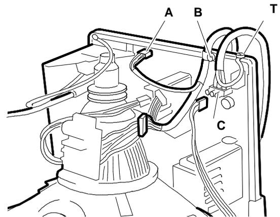
Fig. 4-10 Signals cable and power cable disconnection
