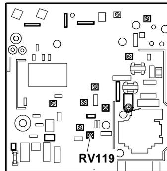
Fig. 4-23 Distortion (pincushion) adjustment
