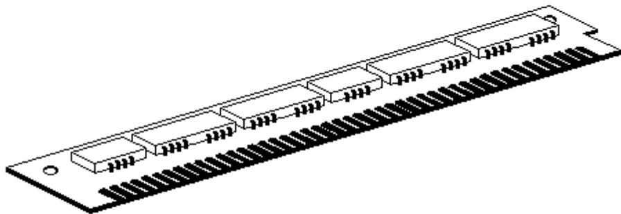
Figure 7-9. Optional 512 Kbyte Memory Module
