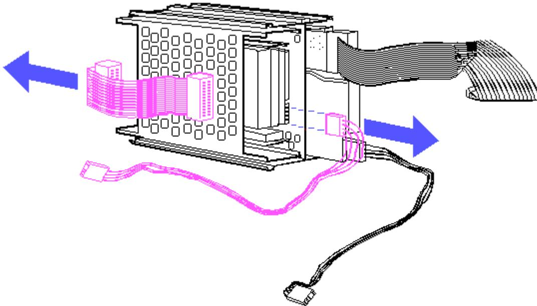
Figure 8-44. Disconnecting the Fixed Disk Drive Cables
