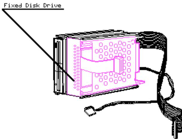
Figure 8-43. Fixed Disk Drive Position 2 Location
