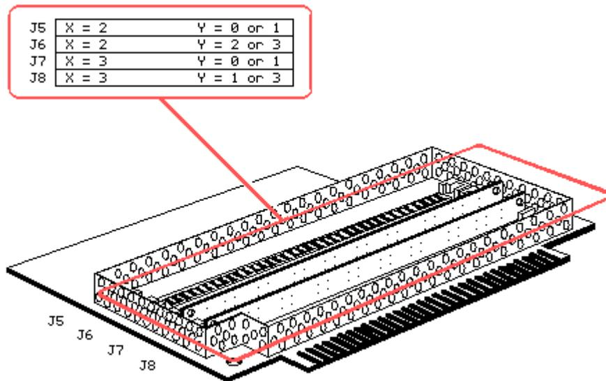
Figure 6-2. 1 to 2 Megabyte Memory Expansion Board Error Map
