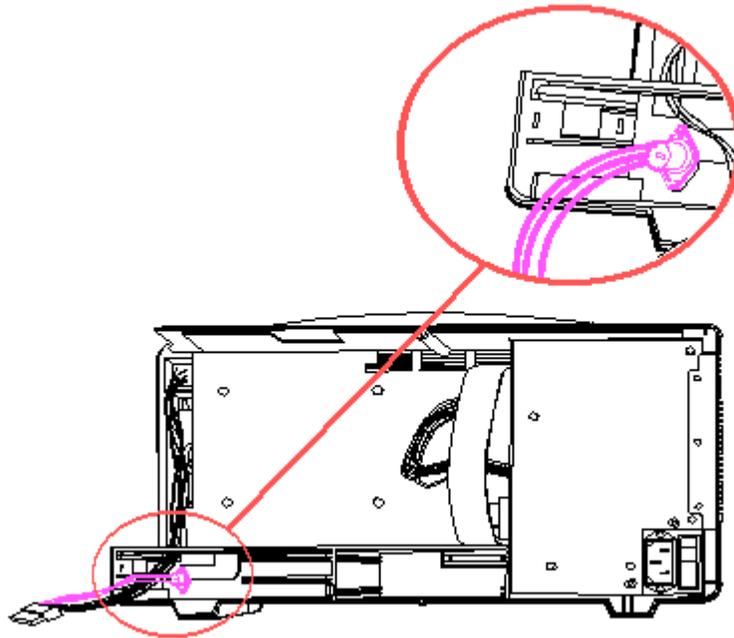
Figure 8-59. Keyboard Cable Connector Location
