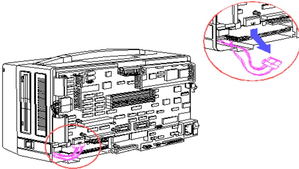
Figure 8-19. Disconnecting the LED/Speaker and Keyboard Cables
