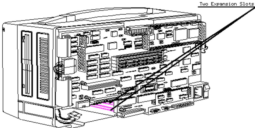
Figure 8-13. Options Compartment with Two Expansion Slots
