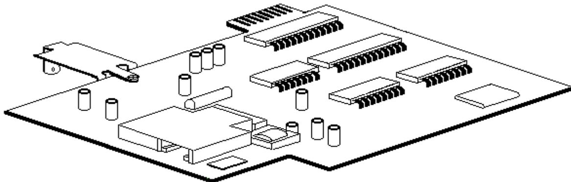
Figure 7-12. Optional COMPAQ 1200 Baud Internal Modem
