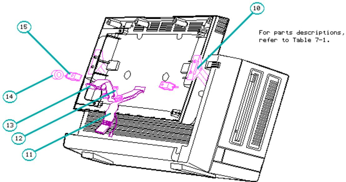
Figure 7-2. Display Enclosure Assembly (Items 10 - 15)
