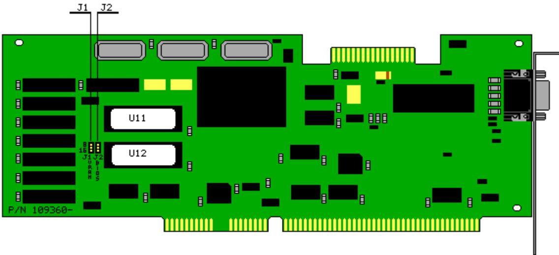
Figure 9-5. Video Graphics Controller Board (Assy No. 109360)
