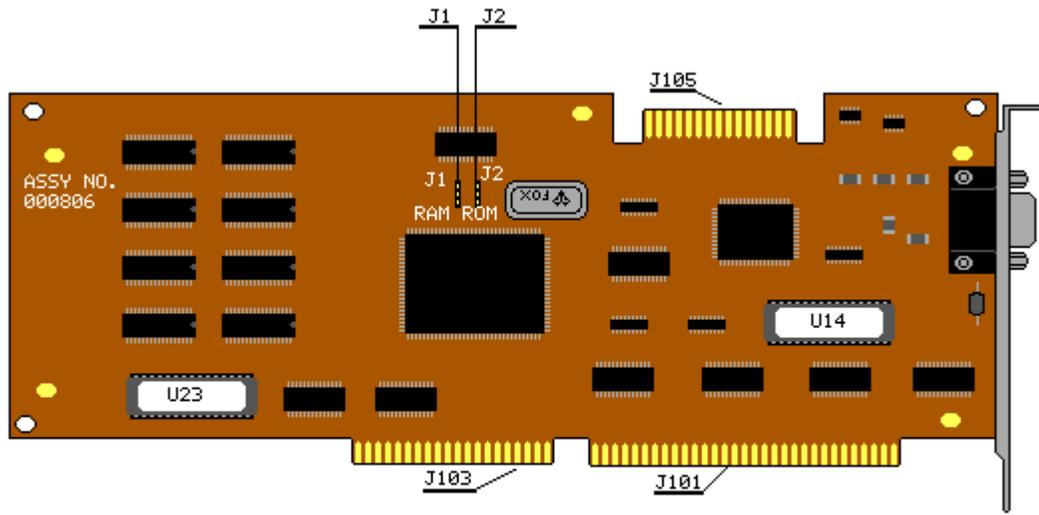
Figure 9-6. Video Graphics Controller Board (Assy No. 000806)
