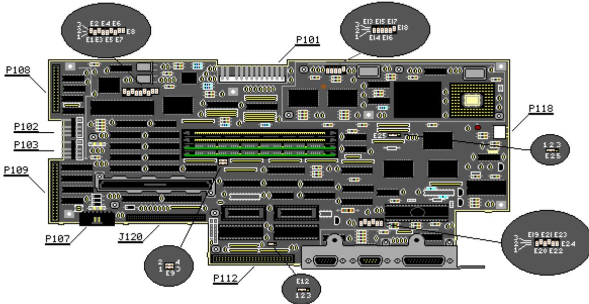
Figure 9-1. System Board Jumper Locations (Assy No. 000510)
