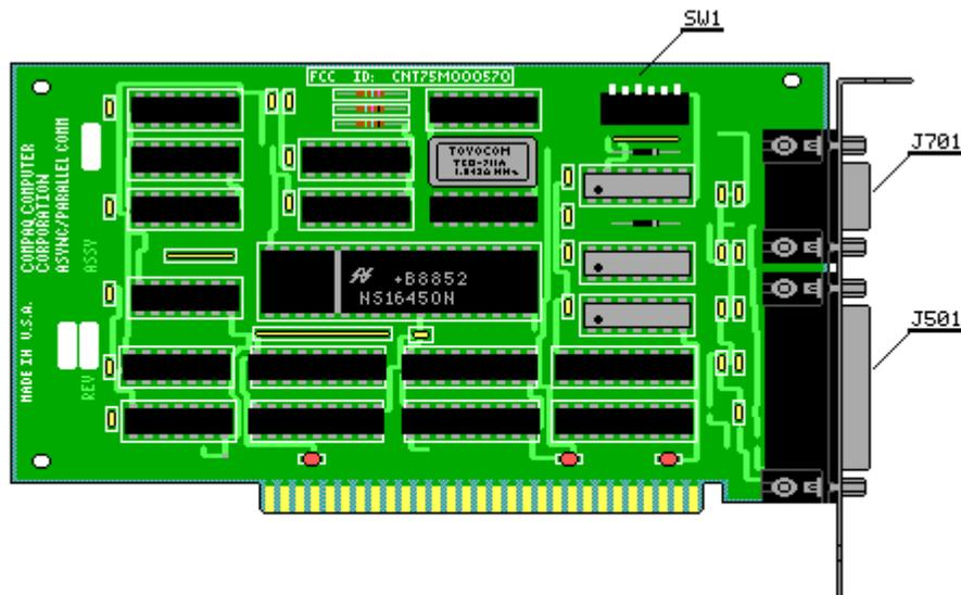
Figure 9-4. Serial/Parallel Interface Board (Assy Nos. 000570 and 000990)
