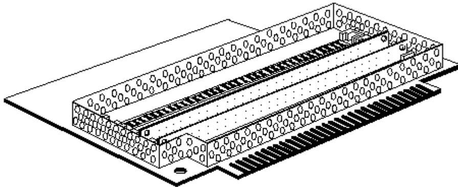
Figure 7-8. Optional 1 to 2 Megabyte Memory Expansion Board
