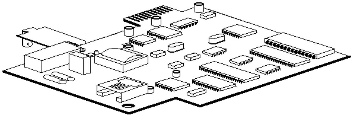
Figure 7-13. Optional COMPAQ 2400 Baud Internal Modem
