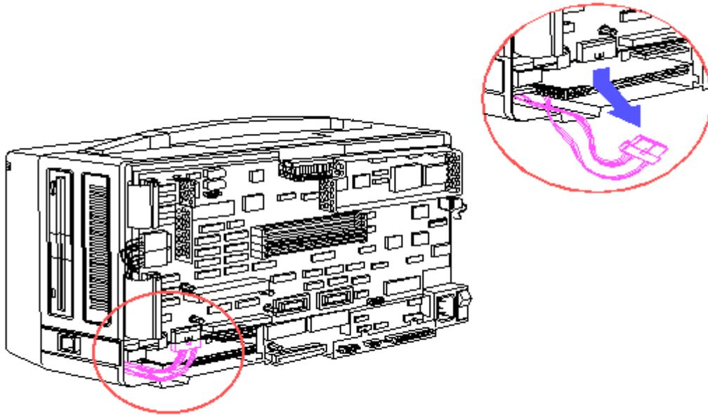
Figure 8-22. Disconnecting the LED/Speaker and Keyboard Cables
