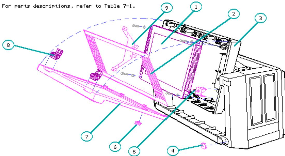
Figure 7-1. Display Enclosure Assembly (Items 1 - 9)
