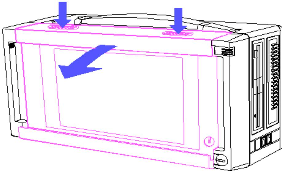
Figure 8-69. Unlatching the Display Enclosure
