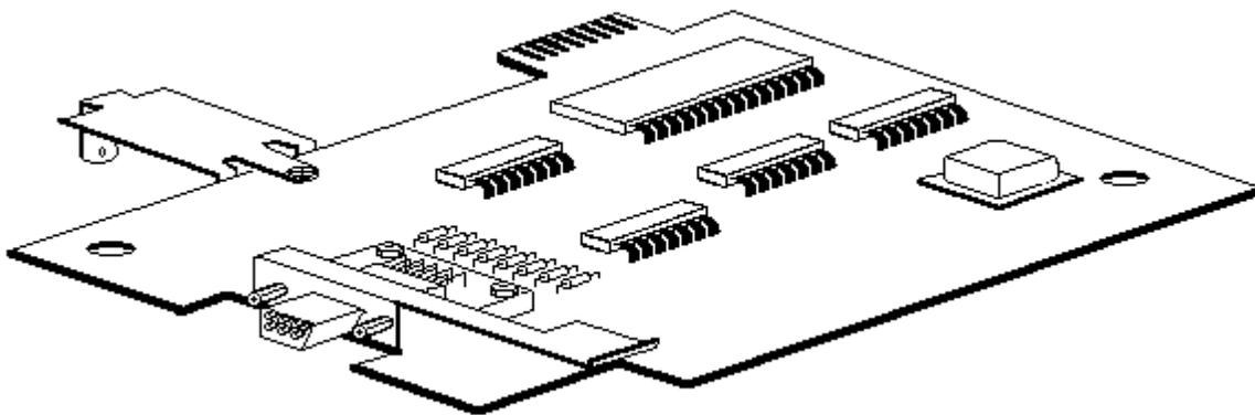
Figure 7-14. Optional Second Serial Interface Board (International Only)
