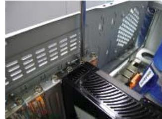
※ If there are power connectors on your card, remember to connect the power cable to them, or the system will not boot. Do not touch the card when it's operating to prevent system instability.
