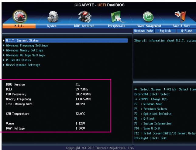
This section provides information on the BIOS version, CPU base clock, CPU frequency, memory frequency, total memory size, CPU temperature, Vcore, and memory voltage.
