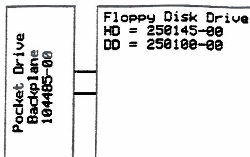
Figure 1-7. Pocket Floppy Disk Drive Components
