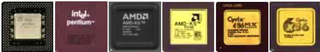
Pentium MMX (P55C) (150MHz-233MHz) Intel Pentium (P54C) (75MHz-200MHz) AMD-K6 (PR166 and faster) AMD-K5 (PR75-PR133) IBM/Cyrix 6x86(MX) (PR166 and faster) IBM/Cyrix 6x86(M1) (PR166 and faster)
