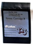
Some JX software is available in handy cartridge form. Cartridge software loads almost immediately, and has the added advantage of not consuming user memory
