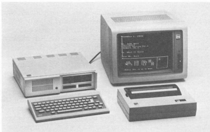
*The PCjr with keyboard and monitor—a complete system*
