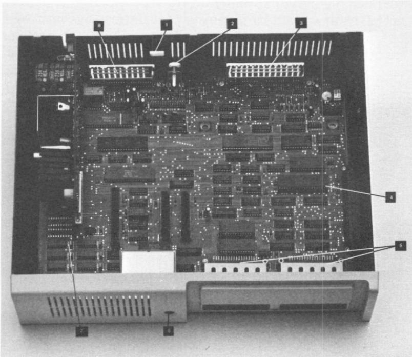
1. Space for internal modem connector and cable. 2. Connector for composite video. 3. Connectors for (l to r): RF modulator (for TV output), light pen, cable for keyboard, reserved by IBM, 1st joystick, 2nd joystick. 4. 8088 CPU. 5. Cartridge slots and connectors. 6. Infrared receiver for keyboard. 7. RAM memory. 8. Connectors for (l to r): audio, transformer power cable, cassette recorder, serial port.
