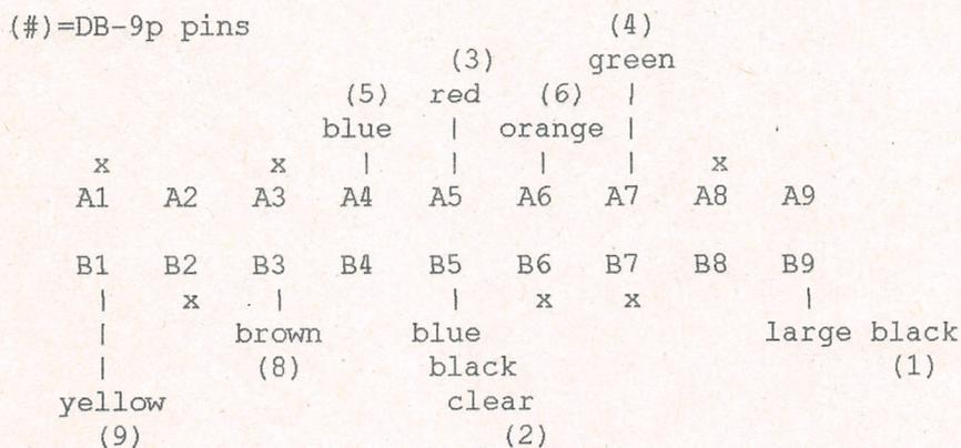
The following are NOT USED (make sure the insulation on these leads is intact so they don't short out - there's power on some of them)
