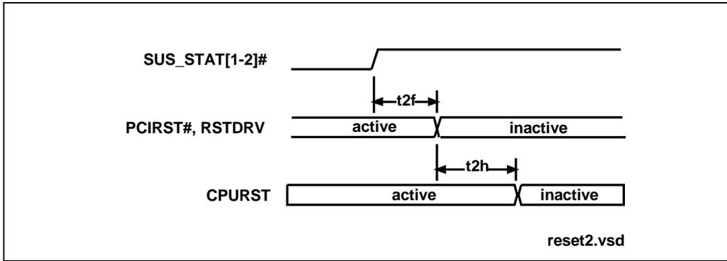
Figure 36. Reset Inactive Timing
