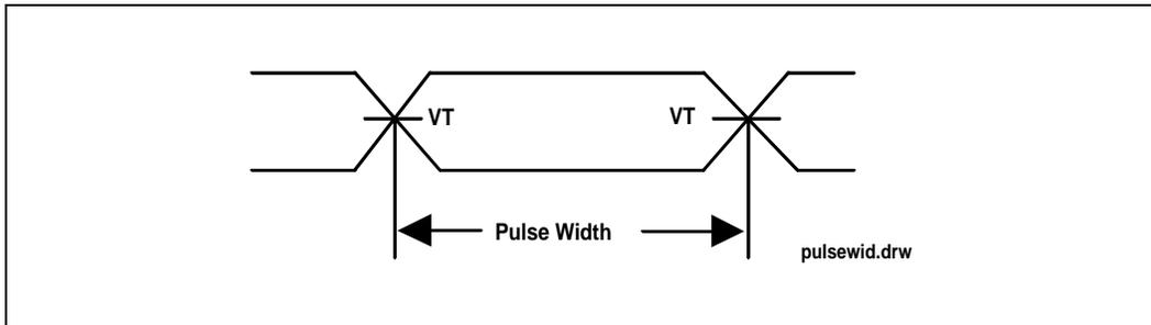
Figure 65. Pulse Width
