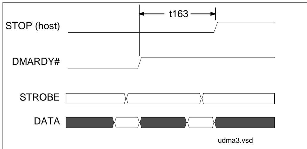
Figure 77. Ultra DMA/33 Receiver Pausing a DMA Burst
