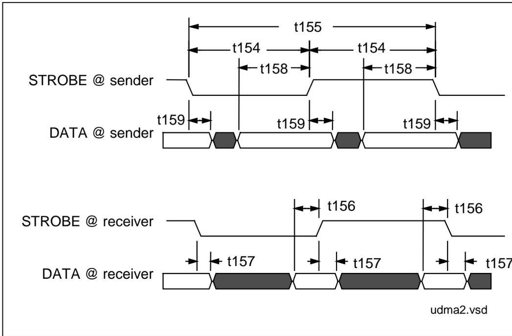
Figure 76. Ultra DMA/33 Sustained Synchronous DMA Burst
