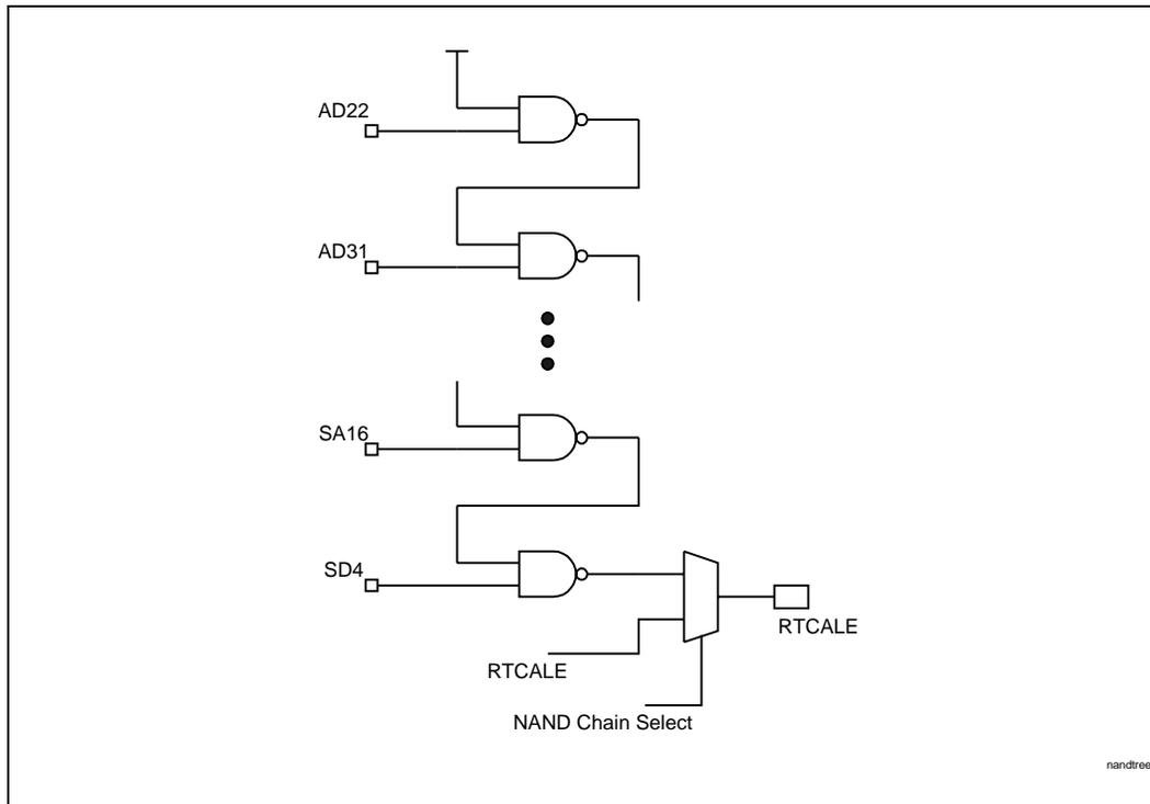
Figure 83. NAND Tree Circuitry (NAND Tree #1 example)
