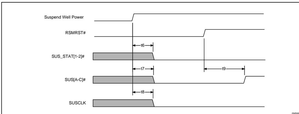
Figure 17. Suspend Well Power and RSMRST# Activated Signals
