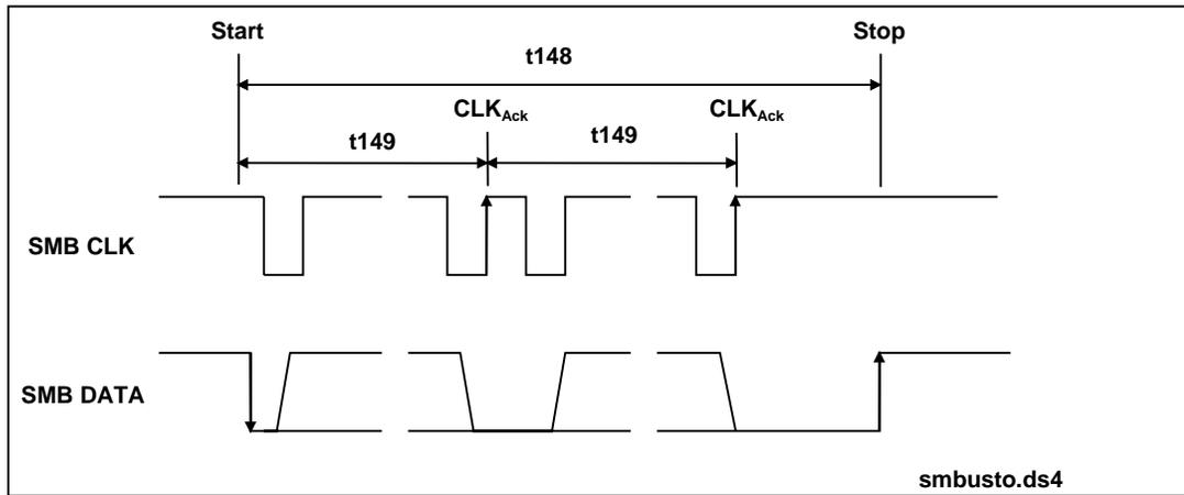
Figure 74. SMBus Timeout Timing
