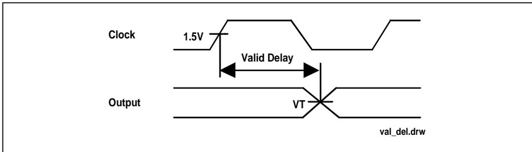
Figure 62. Valid Delay From Rising Clock Edge
