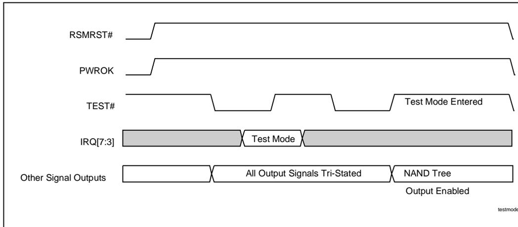
Figure 82. Test Mode Entry (NAND Tree Example)
