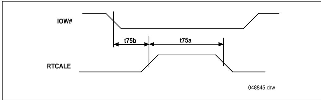
Figure 59. Real Time Clock Timing (RTCALE Generation)
