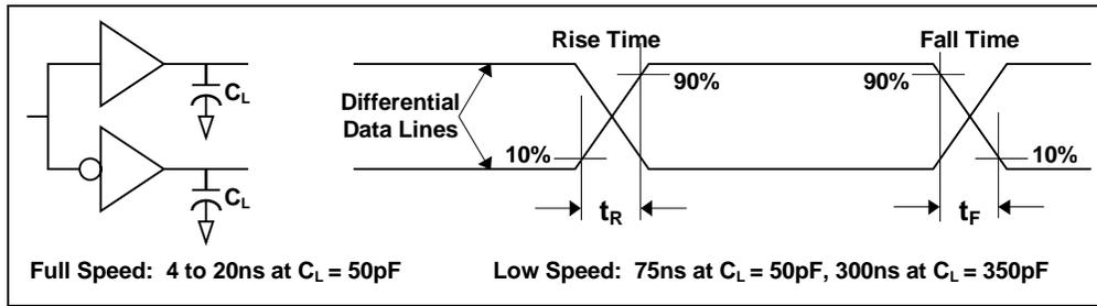
Figure 69. Data Signal Rise and Fall Time
