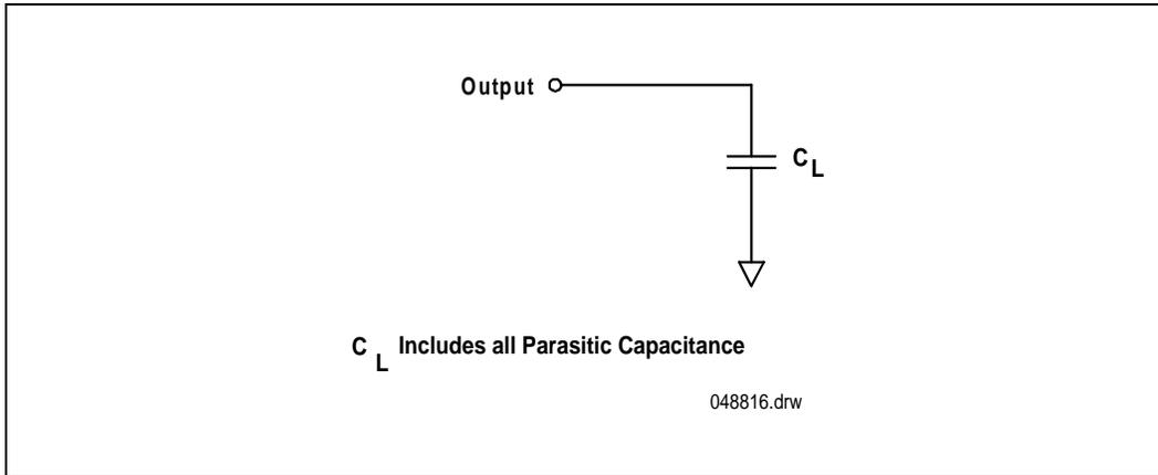
Figure 34. Test Load
