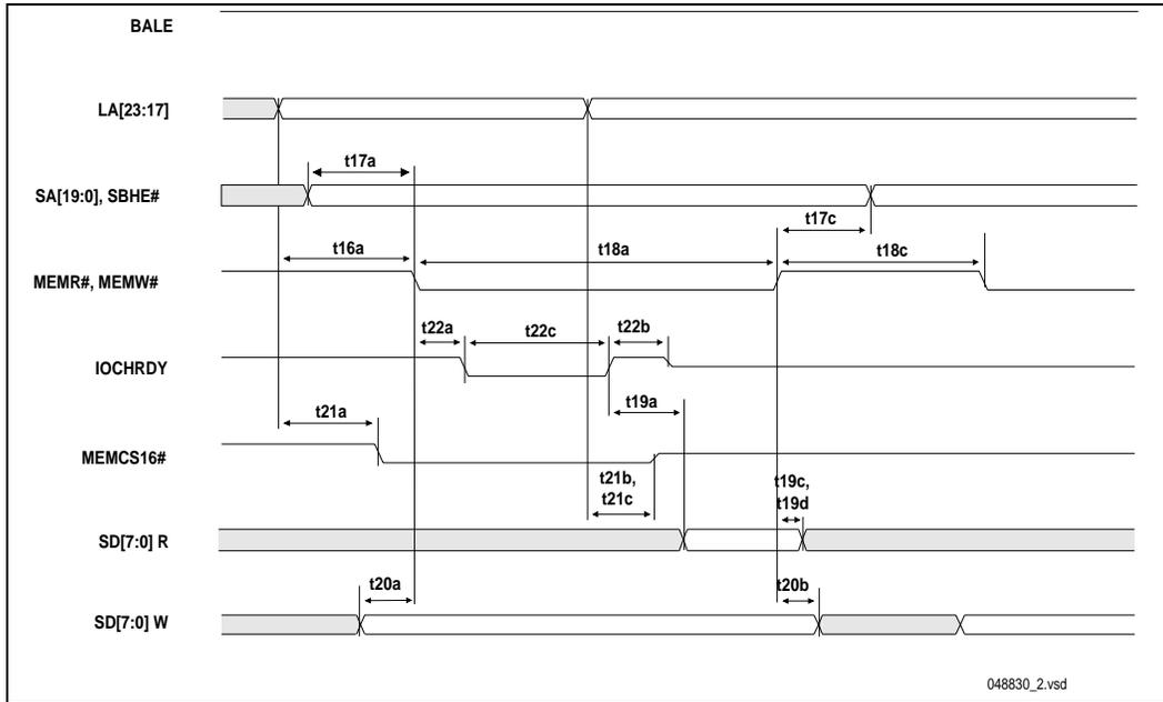
Figure 45. ISA Master Accessing PCI Memory Timing
