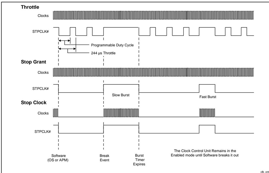
Figure 12. Clock Control Mechanisms (with BURST Enabled)
