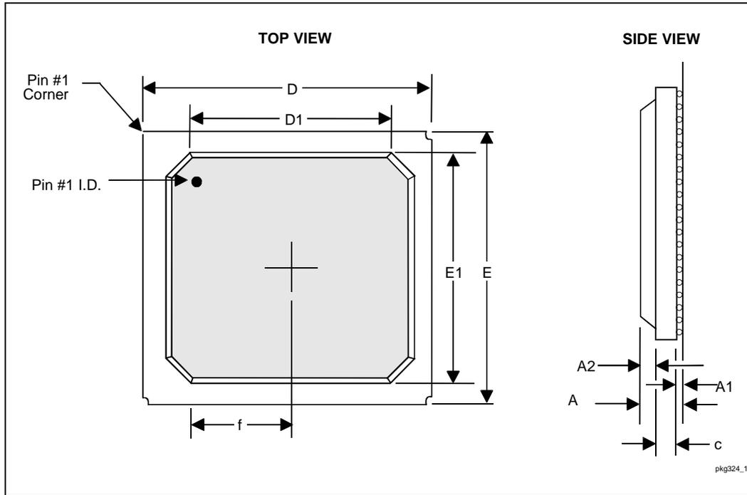
Figure 80. PIIX4E 324-Pin Ball Grid Array (BGA)
