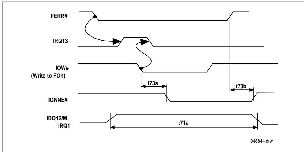
Figure 58. Coprocessor Error and Mouse Support Timing
