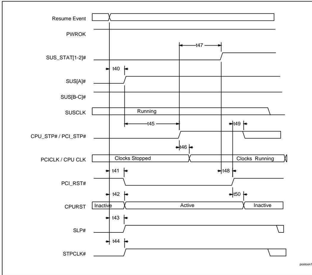
Figure 24. POS to On (w/Processor & PCI Reset)
