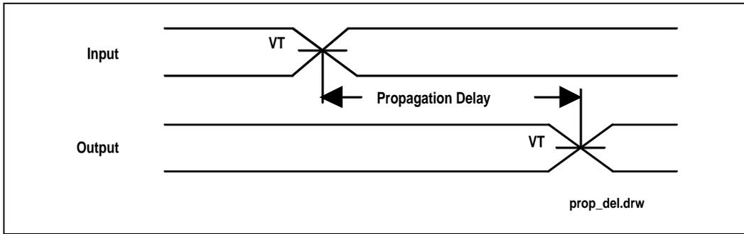
Figure 61. Propagation Delay
