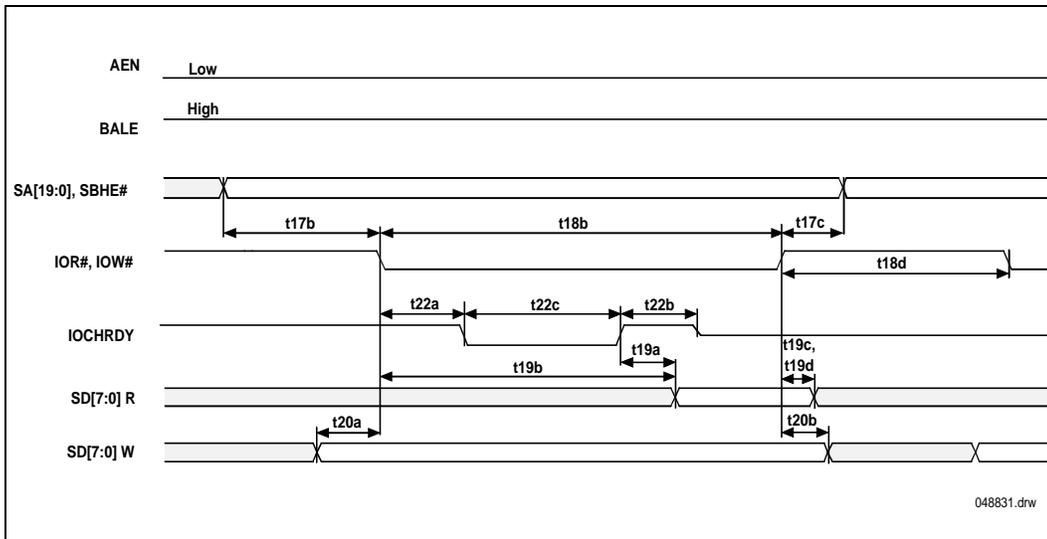
Figure 46. ISA Master Accessing PIIX4E Register Timing
