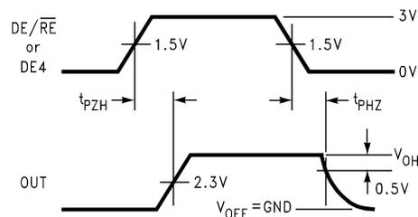
**Figure 6. Driver Enable and Disable Timing ( $t_{PZH}$ ,  $t_{PHZ}$ )**
