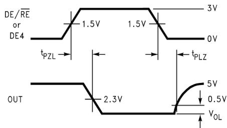
Figure 8. Driver Enable and Disable Timing ( $t_{PZL}$ ,  $t_{PLZ}$ )
