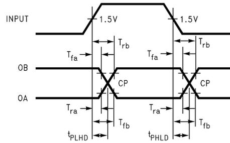
$$T_{CP} = \frac{(T_{fb} \times T_{rb}) - (T_{ra} \times T_{fa})}{T_{rb} - T_{ra} - T_{fa} + T_{fb}}$$
