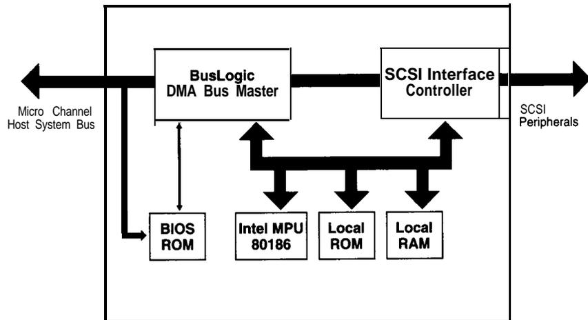
Figure I-1. The BT-646S/BT-646D Block Diagram
