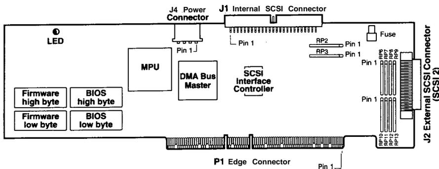
Figure 1-2. The BT-646S/BT-646D Host Adapter Board
