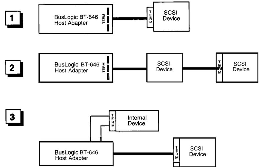
Figure 2-1. SCSI Terminator Configurations
