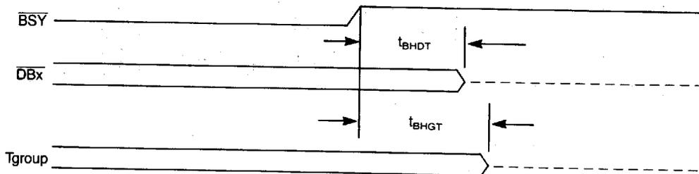
NOTE: Tgroup = signals driven by a Target =  $\overline{\text{I/O}}$ ,  $\overline{\text{C/D}}$ ,  $\overline{\text{MSG}}$ ,  $\overline{\text{REQ}}$
