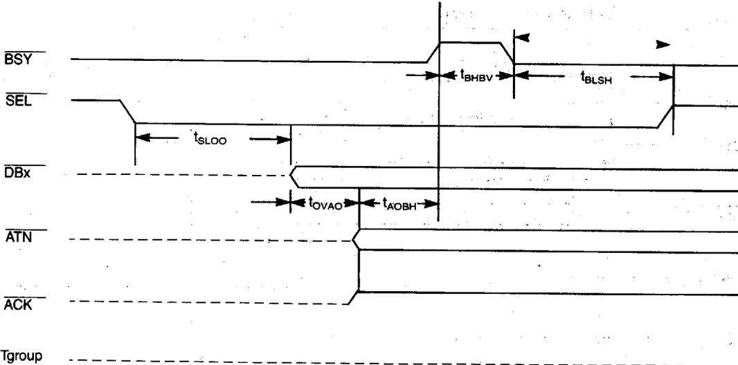
NOTE: Tgroup = signals driven by a Target =  $\overline{I/O}$ ,  $\overline{C/D}$ , MSG, REQ
