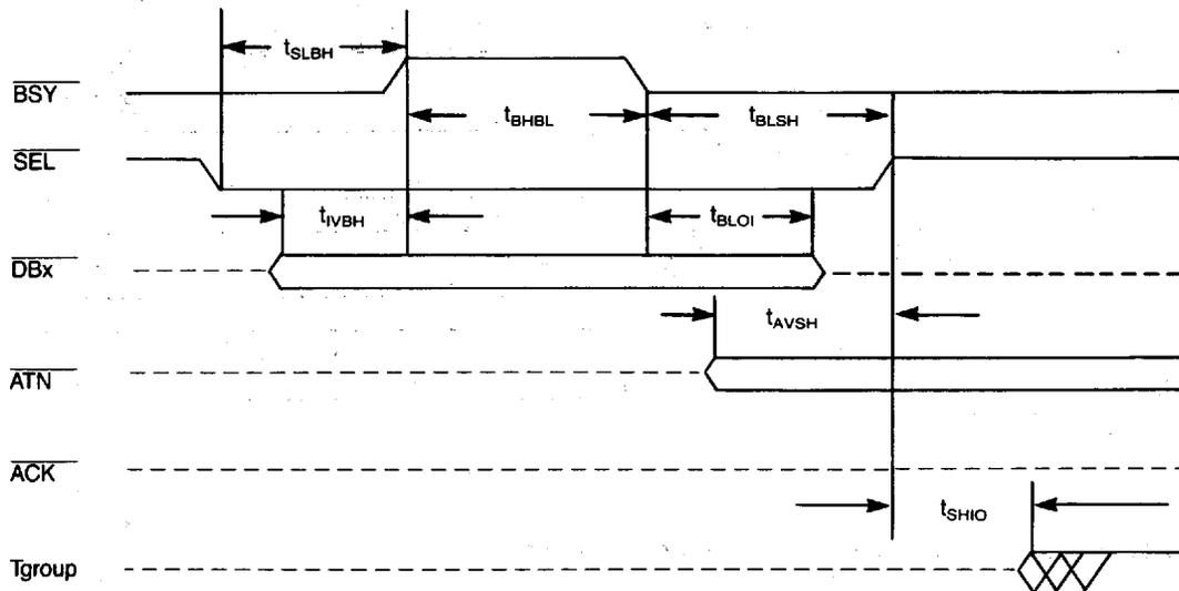
NOTE: Tgroup = signals driven by a Target =  $\overline{I/O}$ , C/D, MSG, REQ
