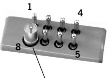
**Note** Pin type for pin 8 differs depending on RF or non-RF configuration (RF pin shown).
