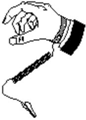
**Note:** With the AC power cord unplugged and the computer's cover removed, the components inside your computer are vulnerable to damage caused by static discharge. Prior to handling any computer hardware, make sure your work area is properly protected against static discharge. There are a number of commercially available static protection devices, designed specifically to help protect your equipment from harmful static discharge.
