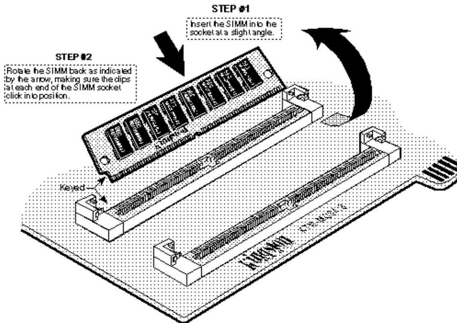
*Figure 2—Installing Memory Modules*
