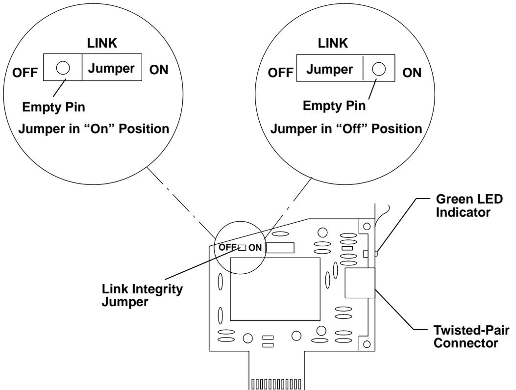
The single green LED on the twisted-pair riser lights when the riser is properly connected to a 10 base T network and the power to the system unit is on. If the green LED does not come on, there could be several possible problems. The twisted-pair cable is defective or not connected, the network is not a 10 base T network, or the Ethernet riser card is not properly installed in the system unit.
