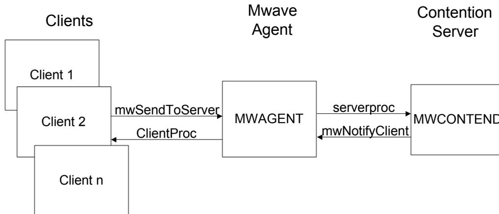
Figure 4-1. Mwave Client-Server Environment
