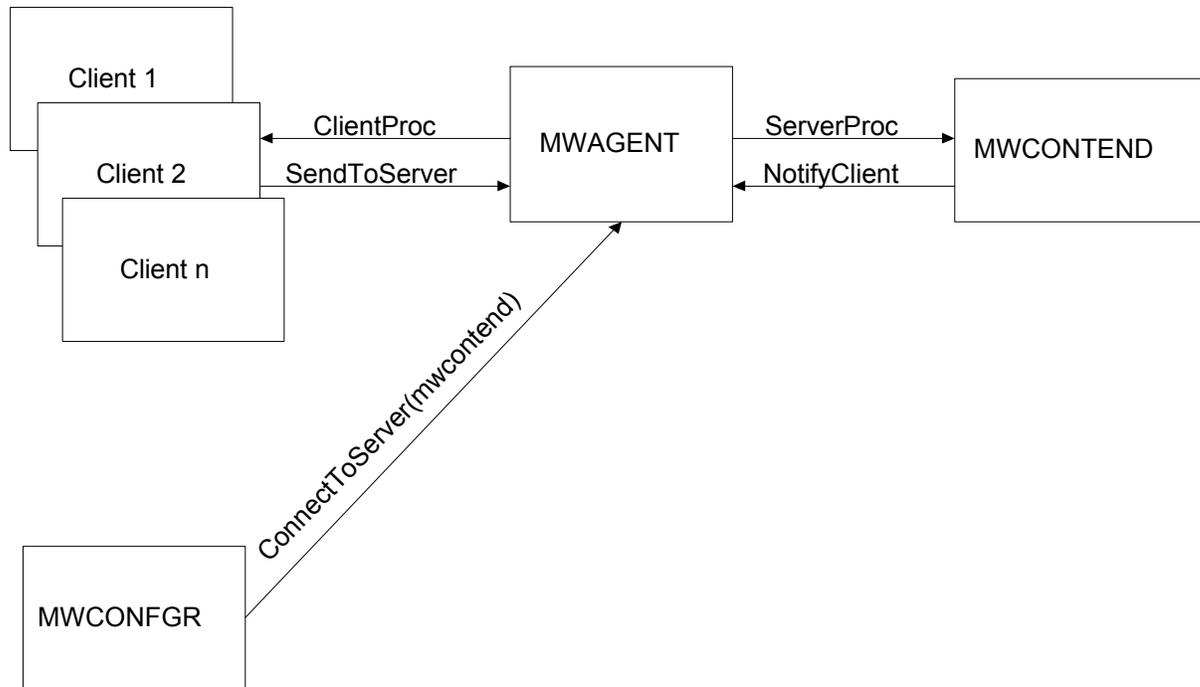
Figure 4-6. MWCONFGR Registers With the Contention Server via MWAGENT
