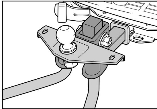
**Clamp-On Bumper Hitch** – This is a temporary hitch that clamps onto the bumper assembly. **DO NOT USE** this type of hitch on any NISSAN vehicle because using it may result in the trailer separating from the towing vehicle. Use of this type of hitch can also damage the towing vehicle.
