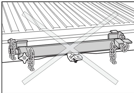
**5th Wheel or Gooseneck Hitch** – Mounted in the bed of a pick-up and designed for heavy-duty applications, these types of hitches are not available from NISSAN but can be purchased from a professional supplier of towing equipment. At this time, Titan is the only NISSAN vehicle approved for 5th wheel and gooseneck trailer towing.
