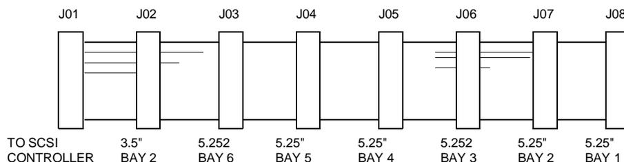
The systems equipped with the 4-connector SCSI cable can configure a second HDU in 5.25" bay 2 (the mechanical support for this bay is already installed at the factory) and a removable SCSI peripheral in 3.5" bay 2 (DAT) or in 5.25" bays 5 or 6.
