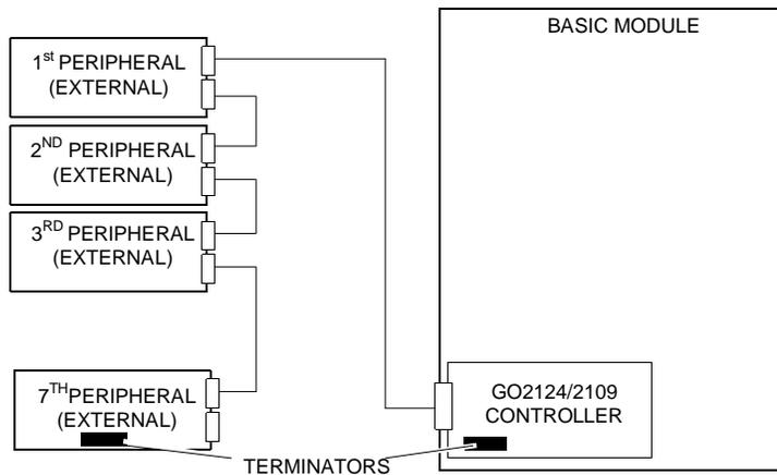
In the case of connection to external SCSI peripherals, excluding the PEM, to the onboard SCSI controller that handles the internal peripherals, the terminator must be disabled from the controller and be present on the last external peripheral connected to the system and on the primary HDU. This type of connection reduces the transfer rate on the SCSI channel from 10 to 5 MB/sec.
