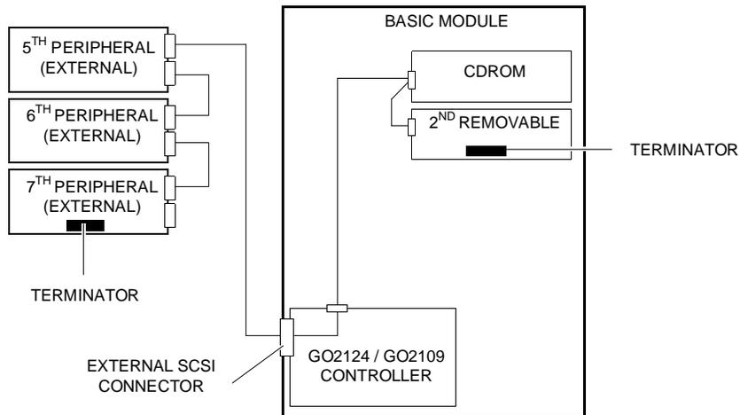
In case internal Wide HDUs are connected to the optional GO2109 SCSI controller that also handles the internal removable peripherals, the terminator must be disabled from the controller and must be present on the system first HDU and on the last internal removable peripheral.
