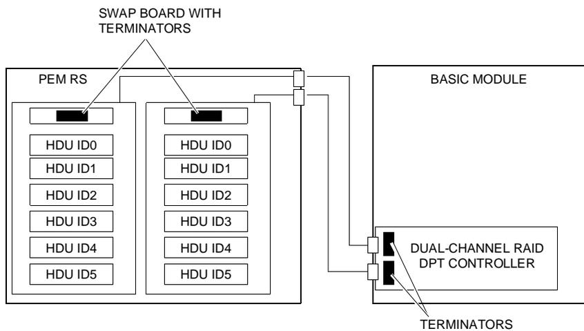
In case external SCSI peripherals, excluding the PEM, are connected to the optional GO2124 or GO2109 SCSI controller that also handles the internal removable peripherals, the terminator must be disabled from the controller and be present on the last external peripheral connected to the system and on the last internal removable peripheral. This type of connection reduces the transfer rate on the SCSI channel from 10 to 5 MB/sec.
