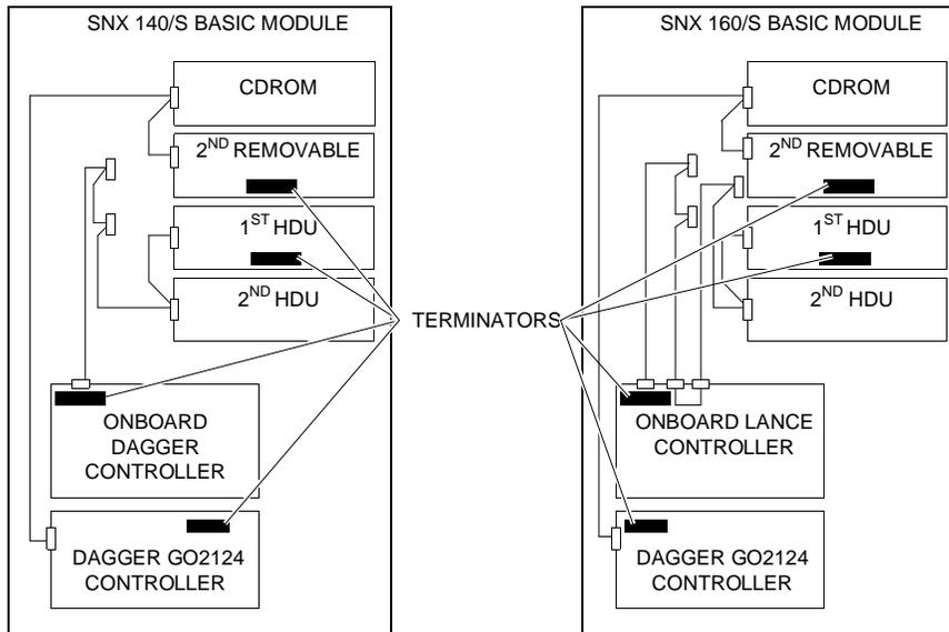
In the case of connection to external SCSI peripherals, excluding the PEM, to a GO2124 or dedicated GO2109, the terminator must be present on the controller and on the last external peripheral connected to the system.
