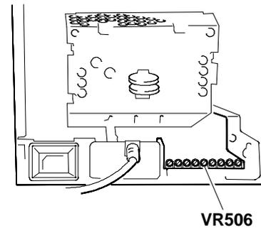
Fig. 10-18 Data area centering adjustment inside the bezel
