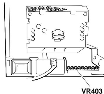
Fig. 10-21 Vertical width (640x480) adjustment
