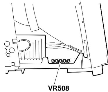
Fig. 10-24 Horizontal width (1024x768) adjustment
