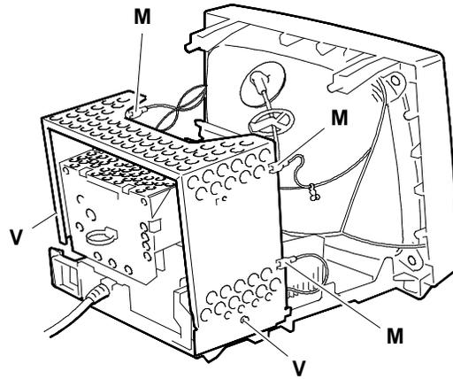
Fig. 10-5 Anti-static metal screen removal
