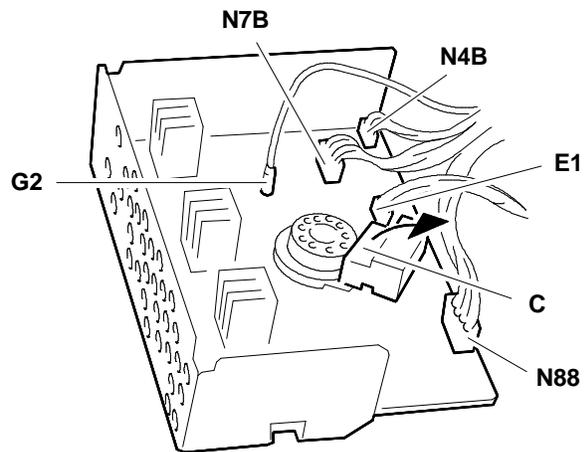
Fig. 10-7 Disconnection of video pre-amplifier board cables
