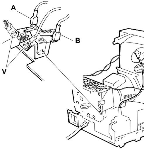
Fig. 10-8 Cable disconnection from ground tank
