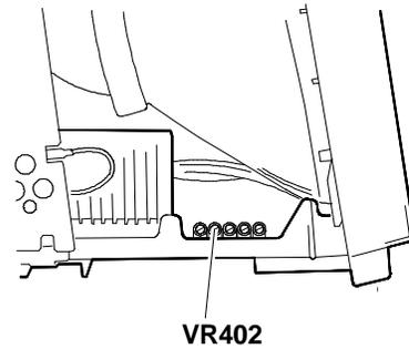
Fig. 10-19 Vertical position adjustment
