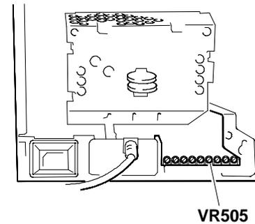
Fig. 10-17 Data area centering adjustment
