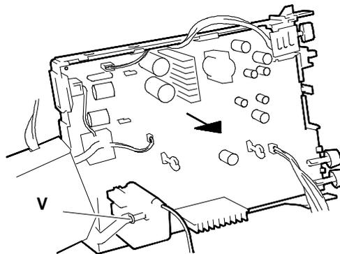
Fig. 10-15 Video motherboard removal
