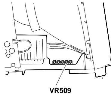
Fig. 10-20 Horizontal width (640x480) adjustment
