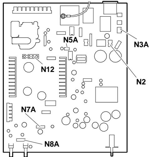
Fig. 10-9 Video motherboard cable disconnection
