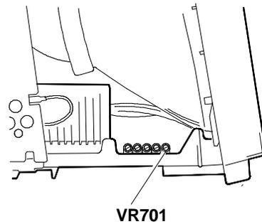
Fig. 10-26 Pincushion distortion adjustment
