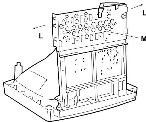
Fig. 10-11 Metal protection (M) removal
