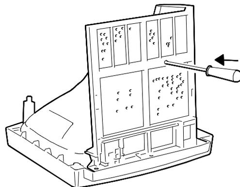
Fig. 10-12 Motherboard fixing pin removal
