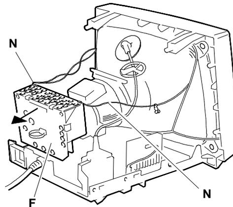
Fig. 10-6 Video pre-amplifier board (F) removal
