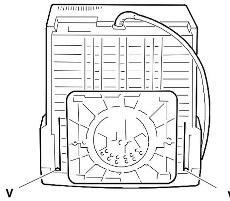
Fig. 10-3 Removal of screws (V) and casing
