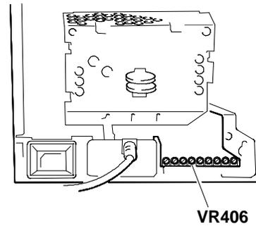
Fig. 10-25 Vertical width (1024x768) adjustment
