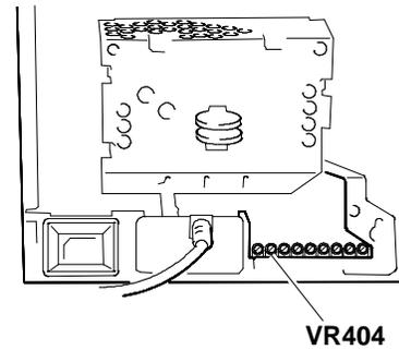
Fig. 10-22 Vertical width (640x400) adjustment
