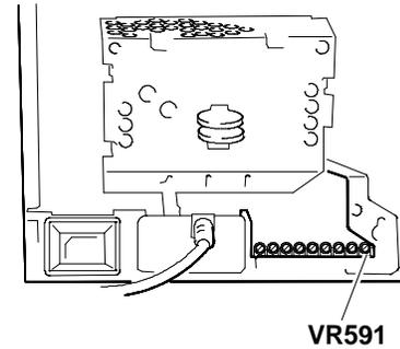
Fig. 10-16 Horizontal centering adjustment
