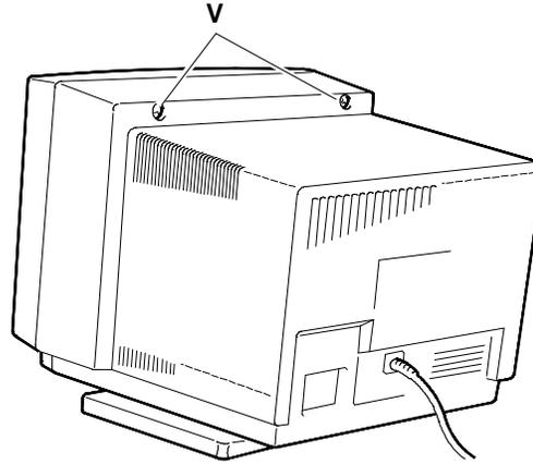
Fig. 10-2 Position of casing screws (V)
