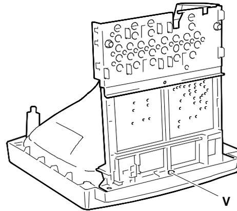
Fig. 10-10 Position of screw that fixes motherboard support structure to video casing
