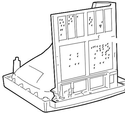
Fig. 10-14 Motherboard support removal
