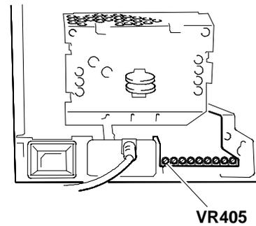
Fig. 10-23 Vertical width (640x350) adjustment
