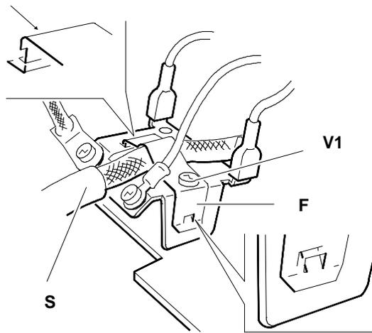
Fig. 10-13 Cable clamp (F) removal
