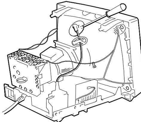
Fig. 10-4 EHT cable disconnection from CRT
