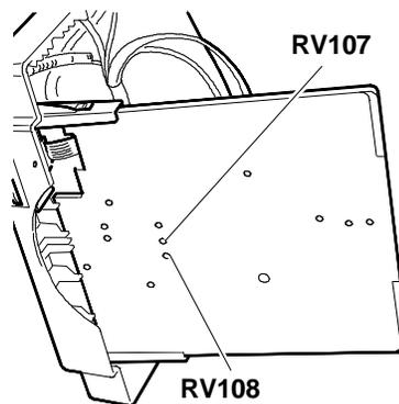
Fig. 19-25 Adjustment of Vertical Width
