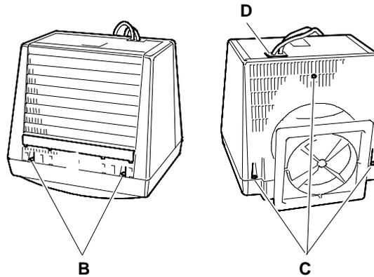
Fig. 19-2 Removal of 6 Screws Securing the Video Cover
