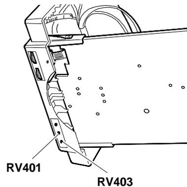
Fig. 19-27 Adjustment of Horizontal and Vertical Width with Resolutions of 600x800 (SVGA) and 1024x768 (XGA)
