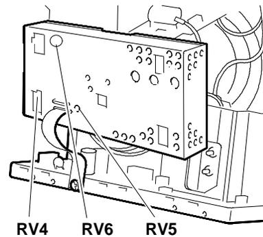
Fig. 19-30 Location of the Potentiometers on the Video Board
