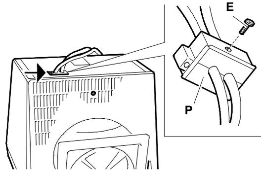
Fig. 19-5 Removal of Cables Support (P)
