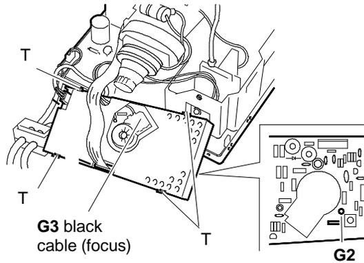
Fig. 19-9 Disconnection of Connections G3 and G2 from Video Amplifier Board
