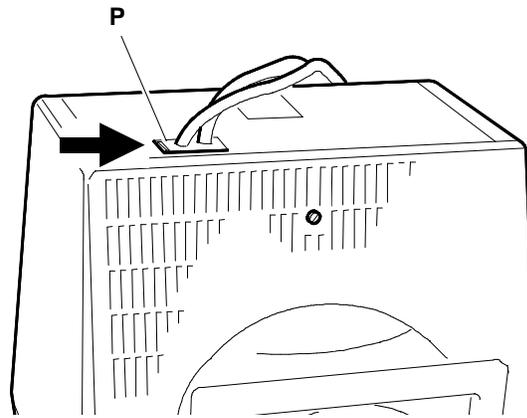
Fig. 19-4 Removal of Video Cables Support
