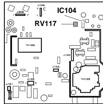
Fig. 19-19 Frequency Adjustment
