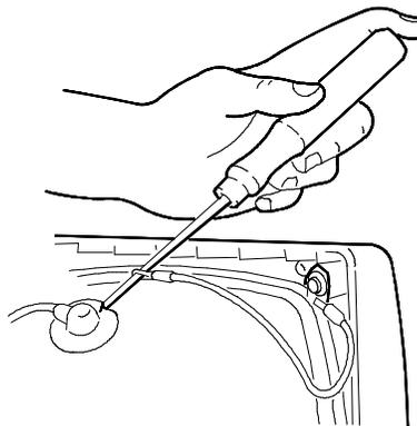
Fig. 19-3 Connection of Screwdriver to Ground
