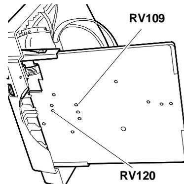
Fig. 19-21 Adjustment of data area dimensions (VGA standard)
