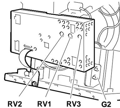
Fig. 19-29 Location of the Potentiometers on the Main Board
