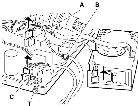
Fig. 19-10 Disconnection of Signals Cable and Power Cord
