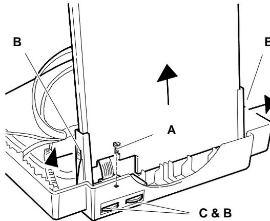
Fig. 19-12 Removal of the Main Board Structure from the Video Casing
