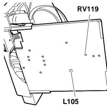
Fig. 19-22 - Adjustment of Pincushion Distortion
