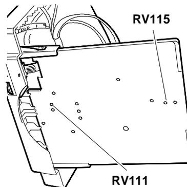
Fig. 19-23 - Adjustment of Vertical Linearity
