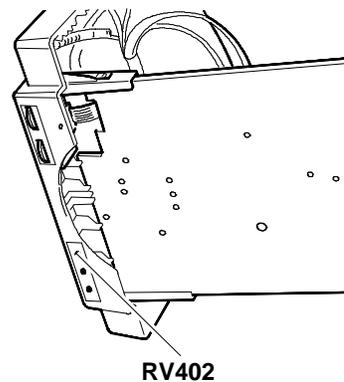
Fig. 19-28 Adjustment of Horizontal Width (VGA standard)
