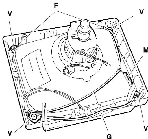
Fig. 19-15 Removal of Cathode Ray Tube
