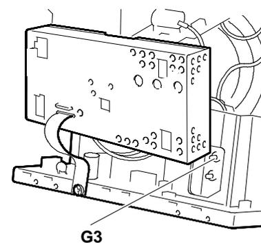
Fig. 19-26 Adjustment of Focus
