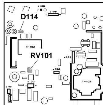
Fig. 19-18 Voltage Adjustment
