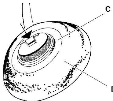
Fig. 19-14 Correct Assembly of CRT Anode
