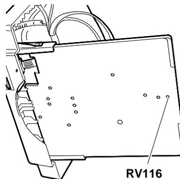
Fig. 19-24 Adjustment of Vertical Centering
