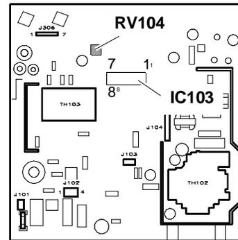
Fig. 19-20 Adjustment of the 31/35 KHz frequency level
