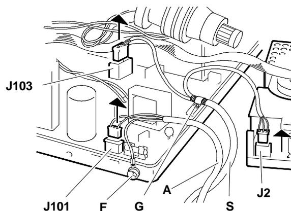
Fig. 19-6 Removal of Video Signals Cable (S) and Power Cord (A)
