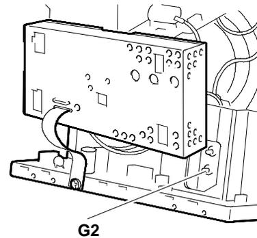
Fig. 19-17 Location of Potentiometer G2 SCREEN
