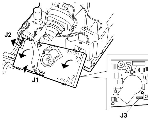
Fig. 19-8 Disconnection of the Cables from the
