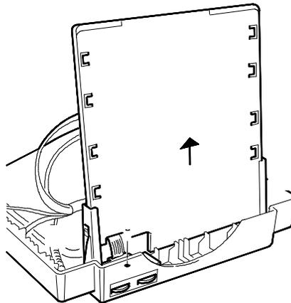
Fig. 19-13 Removal of the Metal Protection Panel from the Solder Side of the Main Board
