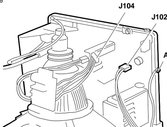
Fig. 19-11 Disconnection of Cables from Main Board
