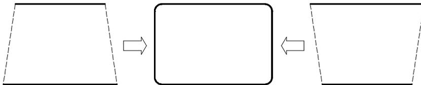
Fig. 27-10 Trapezoidal Distortion Adjustment
