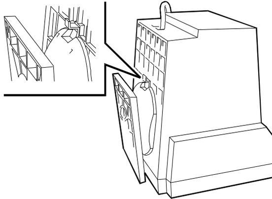
Fig. 31-2 Removal of the Pedestal
