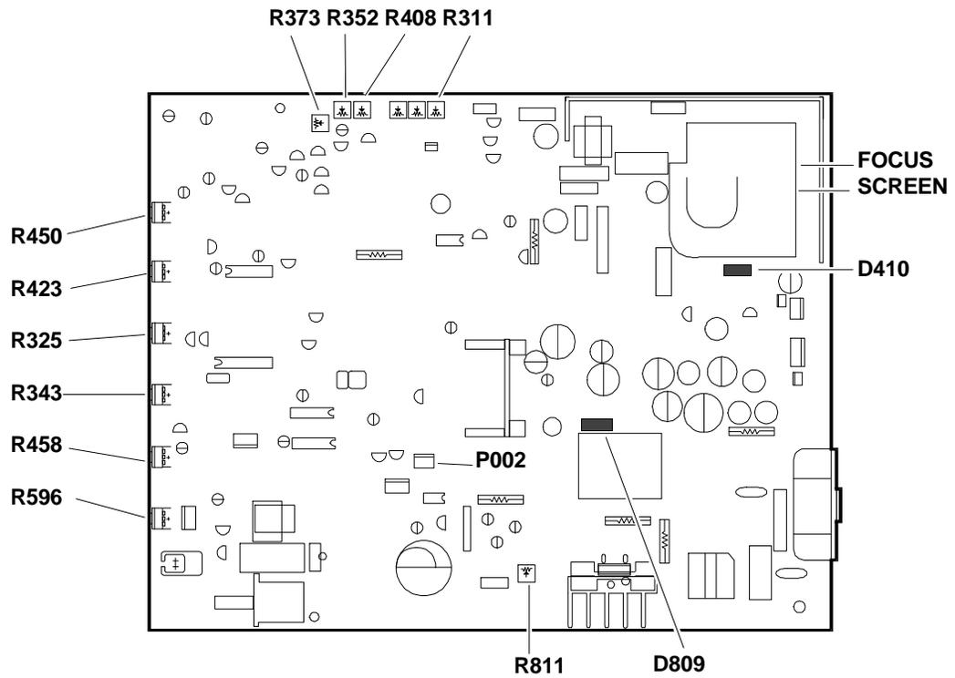
Fig. 31-12 Motherboard Adjustments
