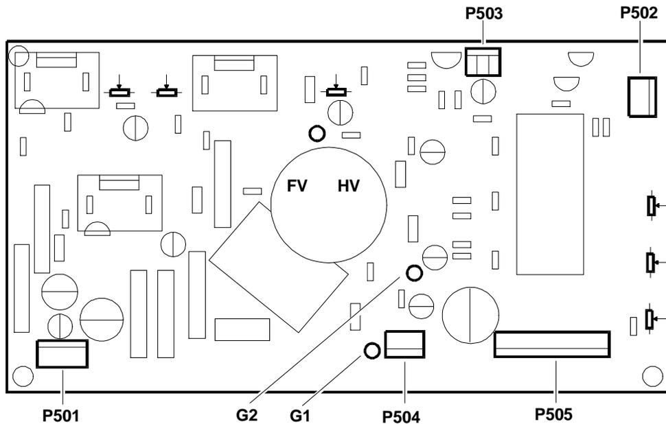
Fig. 31-5 Video Amplifier Board Connectors Location
