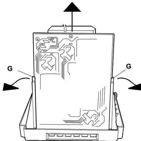
Fig. 31-7 Removing the Motherboard
