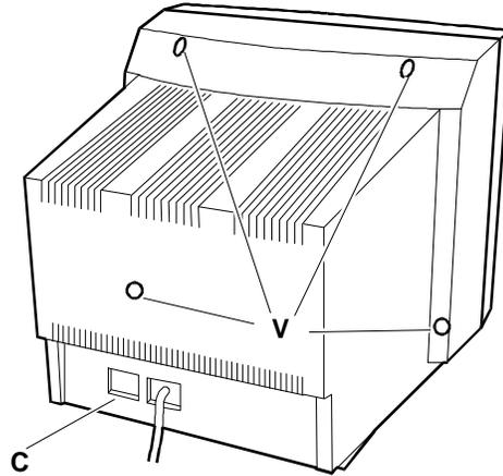
Fig. 31-1 Video Casing Screws Location
