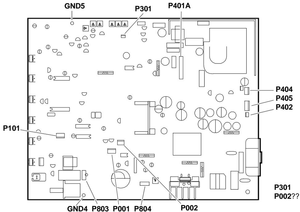
Fig. 31-6 Motherboard Connectors Location
