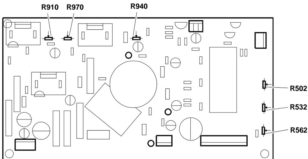
Fig. 31-11 Video Amplifier Board Adjustments
