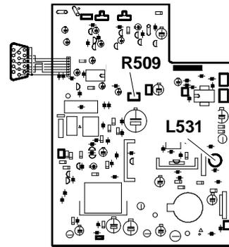
Fig. 6-6 - Horizontal width adjustment
