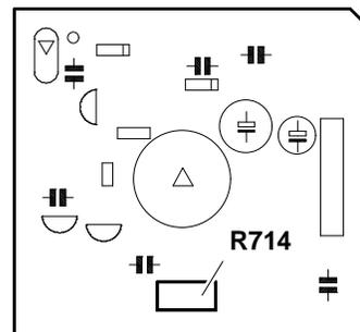
Fig. 6-8 Focus adjustment on video pre-amplifier board
