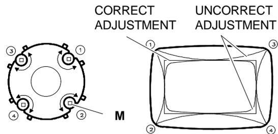
Fig. 6-10 Geometric distortion adjustment
