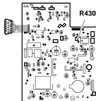
Fig. 6-5 Vertical linearity pre-adjustment
