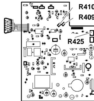
Fig. 6-7 Vertical width adjustment
