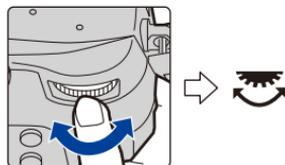
Allows you to set the aperture, shutter speed, and other settings when in **P / A / S / M** modes.
