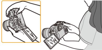
• When not using the monitor it is recommended that you close it with the screen facing inward to prevent dirt and scratches.
