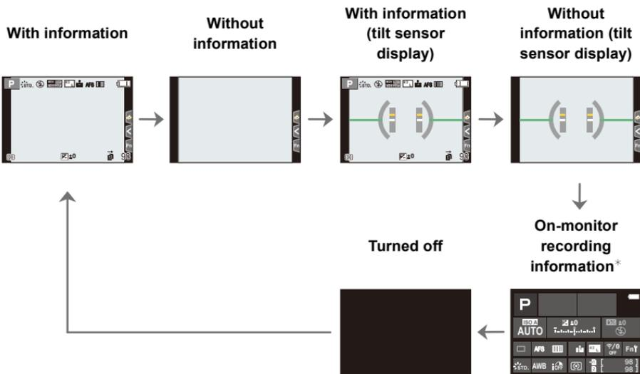
\* When the on-monitor recording information screen is displayed, you can touch the desired item and change its setting directly.
