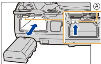
When removing the battery, push the lever **A** toward the arrow and pull out the battery.
