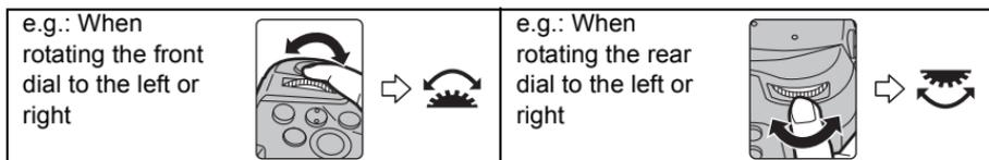
Allows you to set the aperture, shutter speed, and other settings when in **P / A / S / M** modes.
